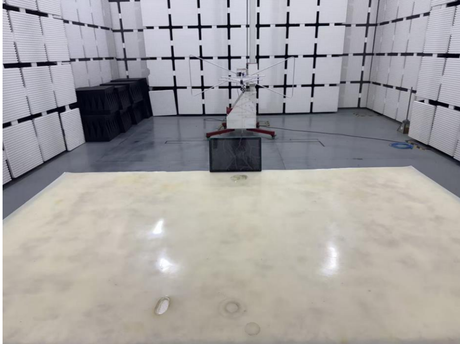
Set-up for Radiated Spurious Emission, Above 1GHz
