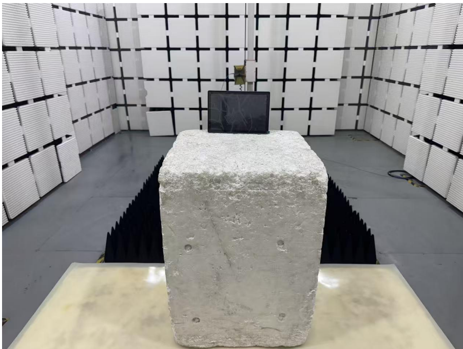
Set-up for Radiated Spurious Emission, Above 1GHz
