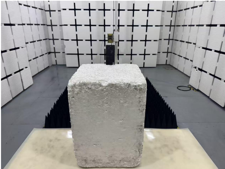
Set-up for Radiated Spurious Emission, Above 1GHz
