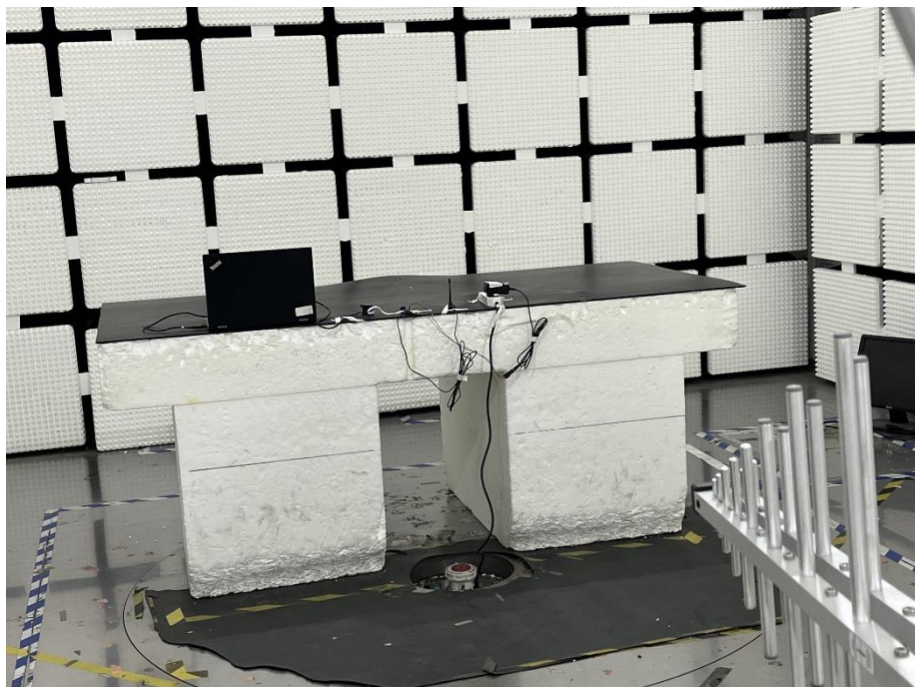
Radiation Emission Test Setup (30MHz to 1GHz)
