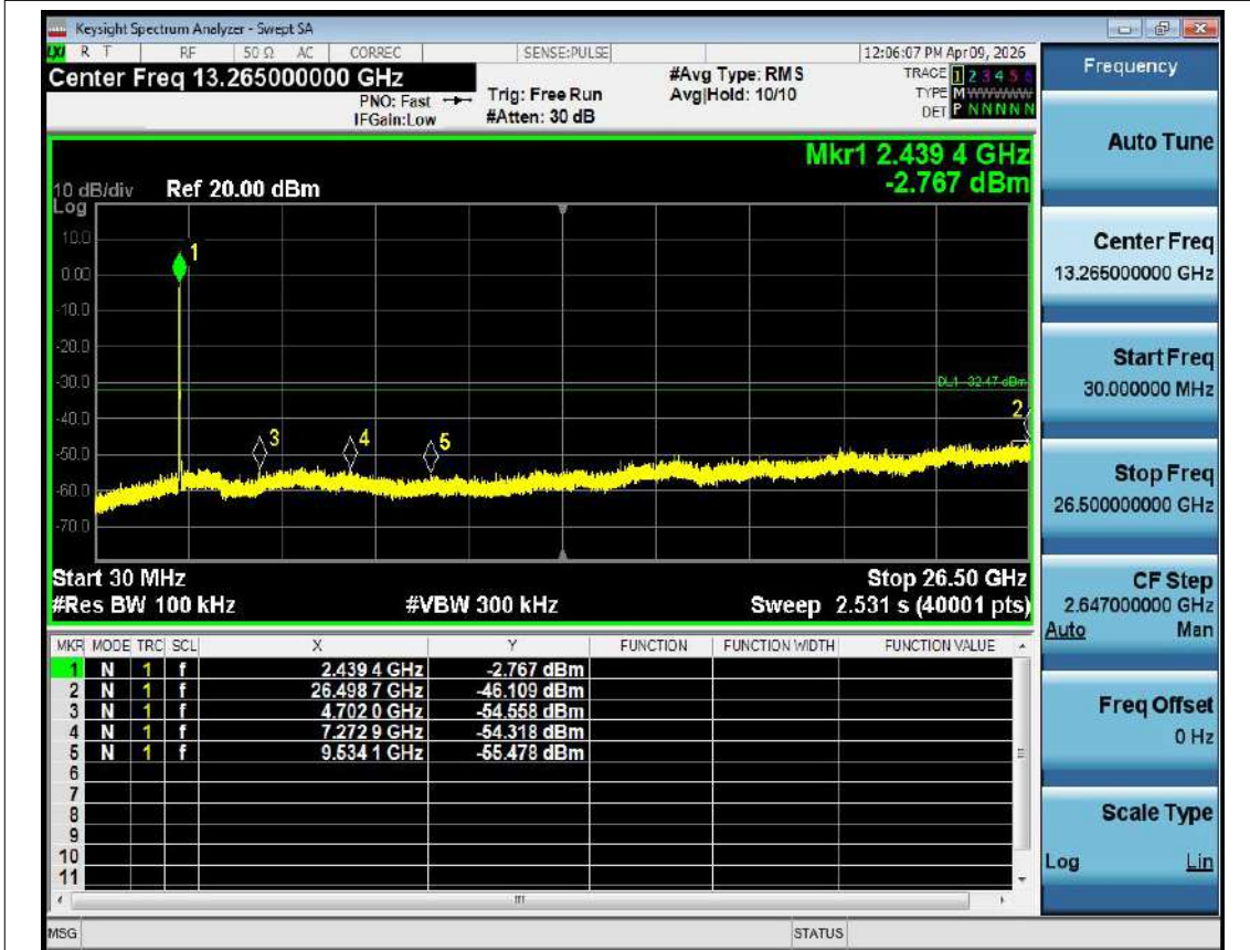
Tx. Spurious NVNT n40 2422MHz Ant1 Emission
