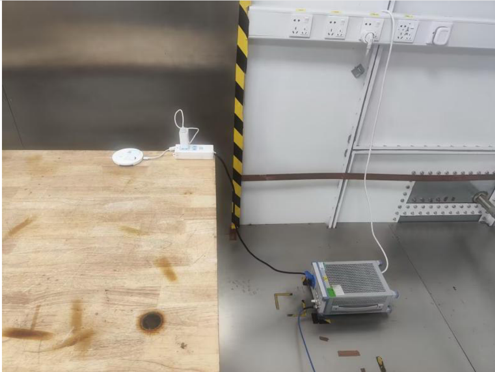
AC Power Line Conducted Emission
