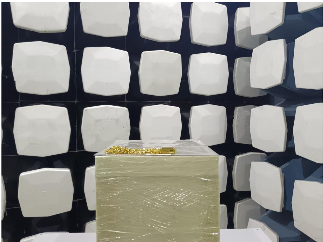
1GHz to 18GHz (The EUT placed at the center of the turntable)
