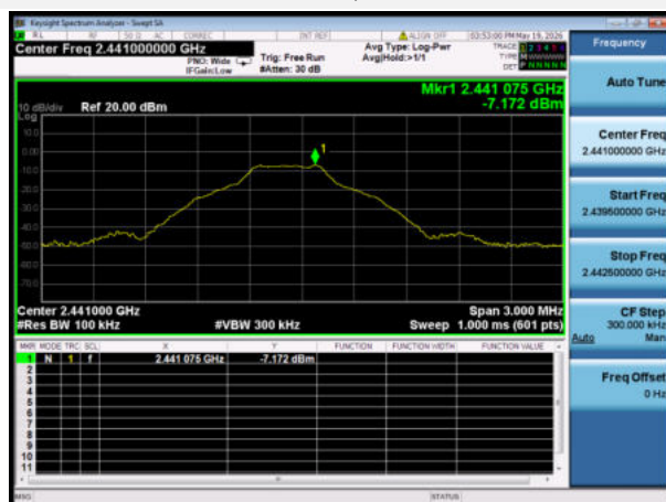
GFSK MIDDLE CHANNEL, CARRIER LEVEL
