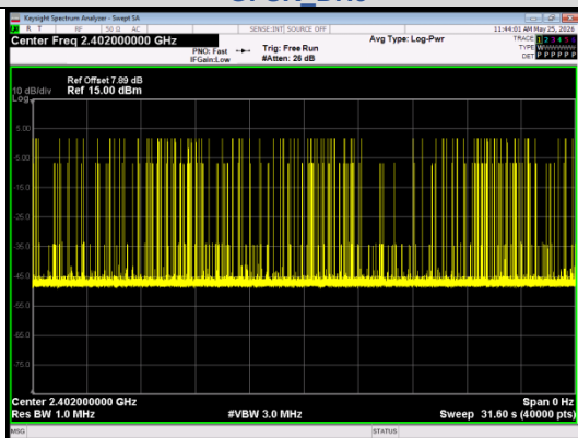
Number of Pulses in 31.6 seconds \pi/4 DQPSK_2-DH5
