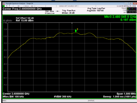
In-Band Reference Level 8DPSK 3-DH1 Channel 78
