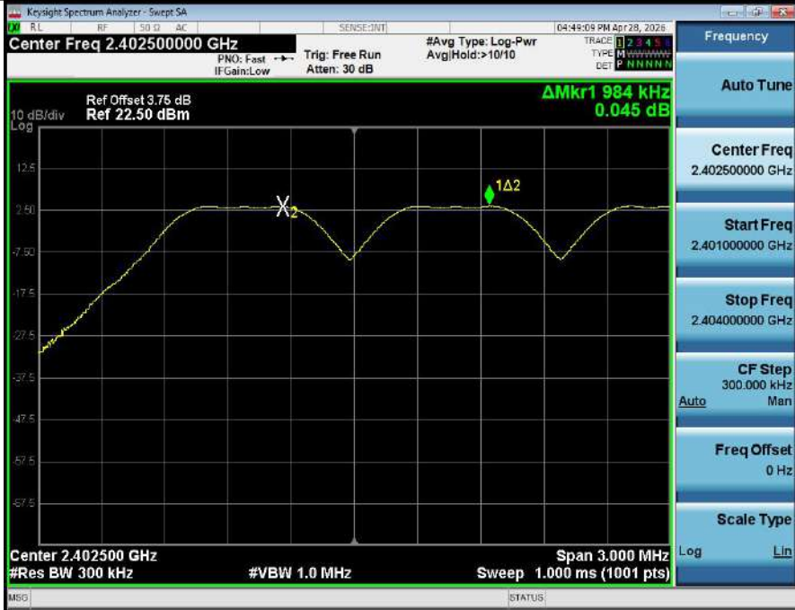
Carrier Frequencies Separation (Hopping) NVNT ANT1 1-DH1 Hopping
