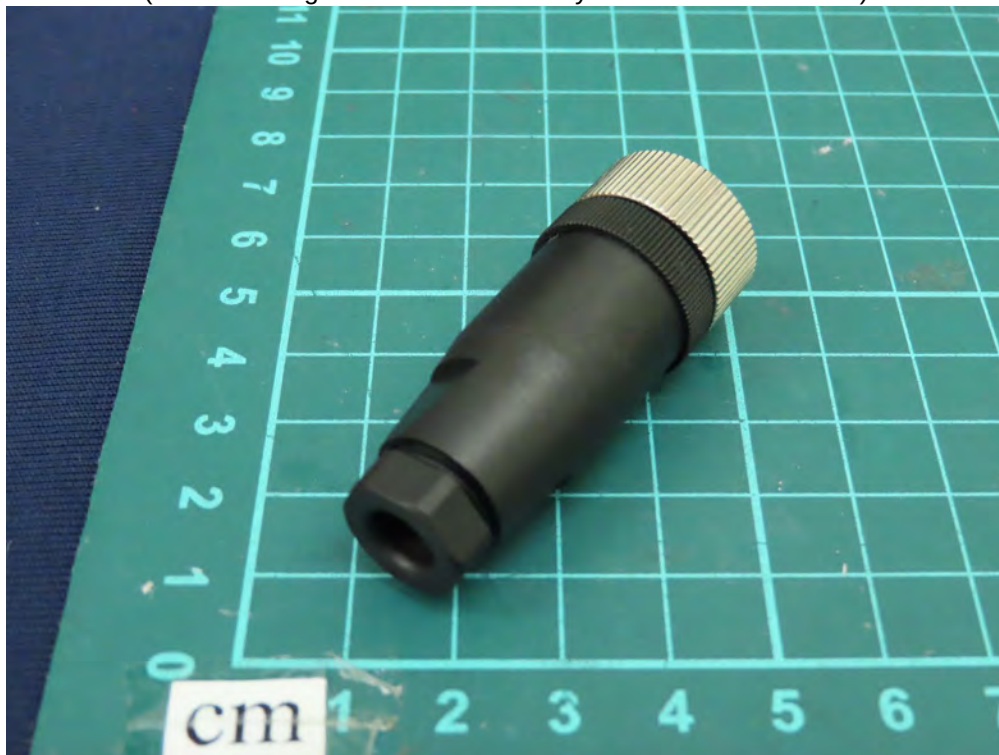
(17) EUT Photo (M12 A Coding 4Pin female Assembly Plastic connector PG7)
