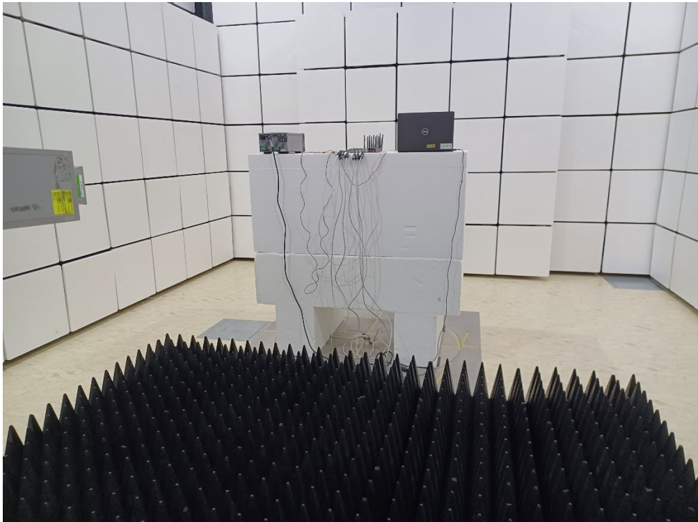
Radiated Test (Above 1 GHz)
