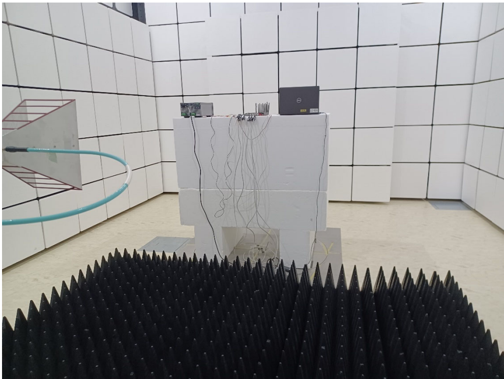
Radiated Test (Above 1 GHz)
