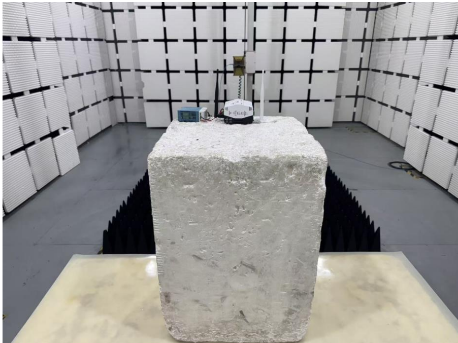
Set-up for Radiated Spurious Emission, Above 1GHz
