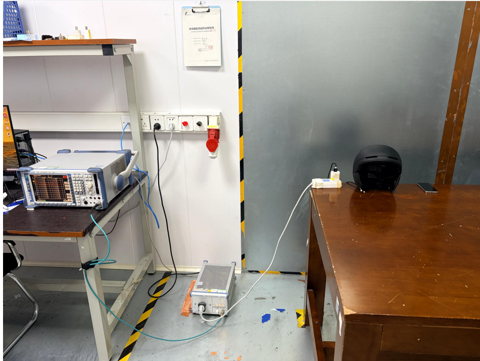
Conducted emissions at AC power line (150kHz-30MHz)
