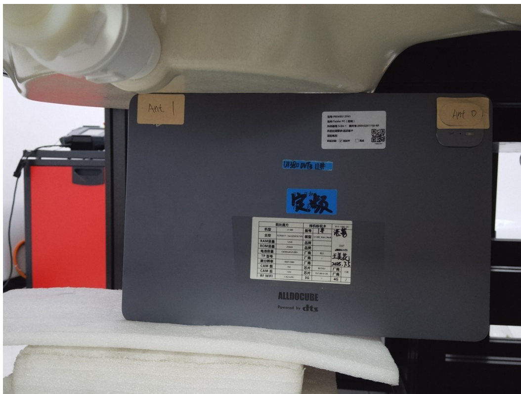
ANT1 Body Top Setup Photo (0 mm)
