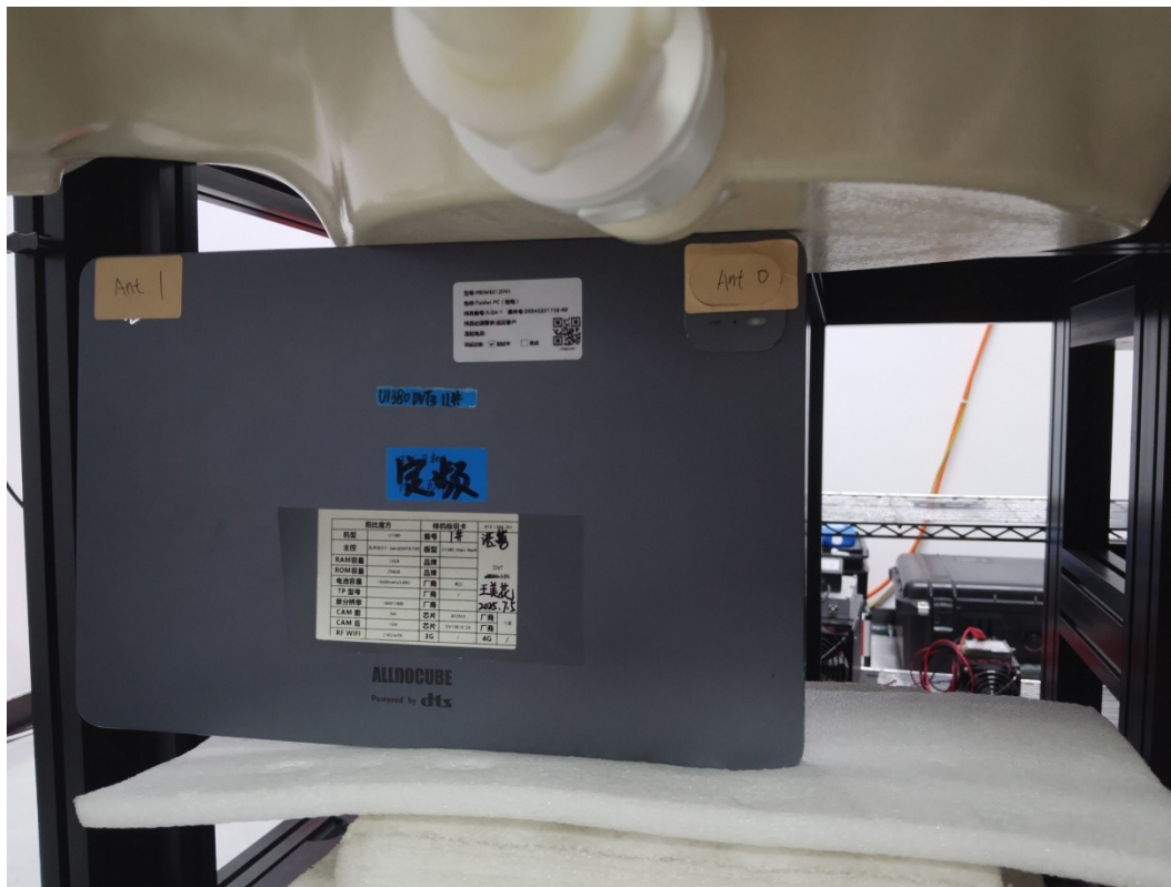
ANT1 Body Top Setup Photo (0 mm)
