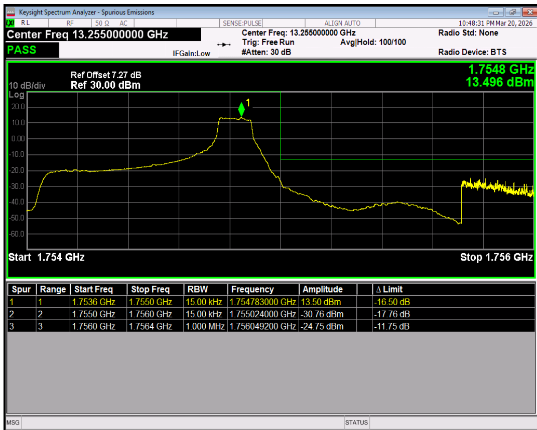
Band4 16QAM BW=1.4MHz Channel=20393 RB Size=6 Position=#0
