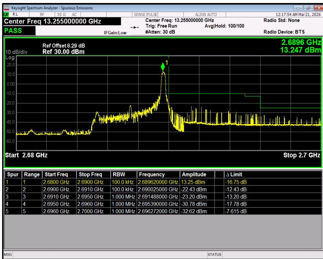
Band41 16QAM BW=5MHz Channel=41565 RB Size=25 Position=#0
