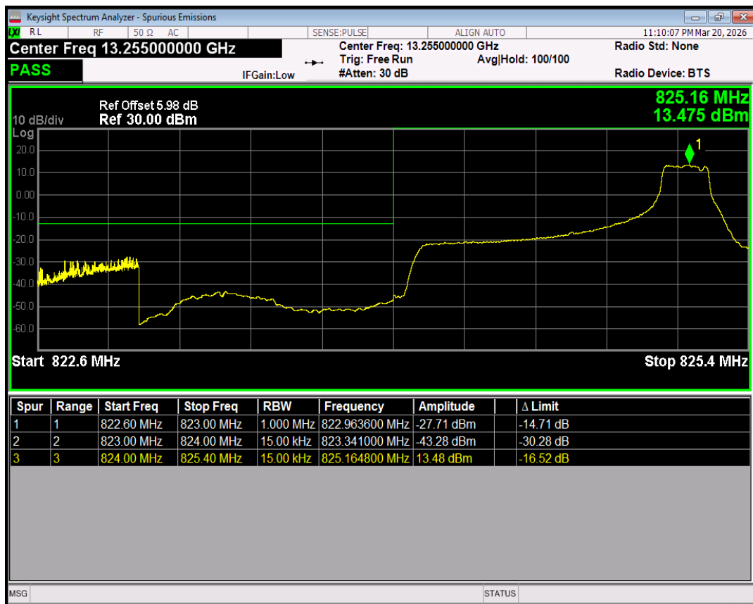
Band5 16QAM BW=1.4MHz Channel=20407 RB Size=6 Position=#0
