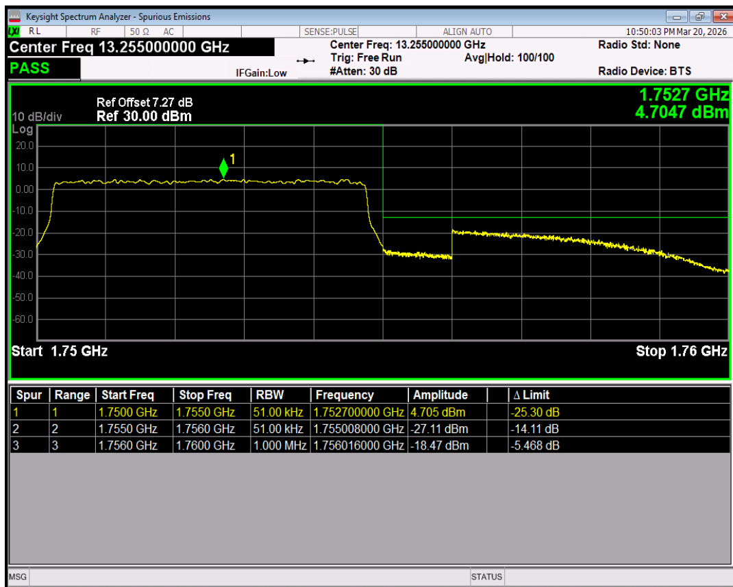
Band4 16QAM BW=5MHz Channel=20375 RB Size=1 Position=#0
