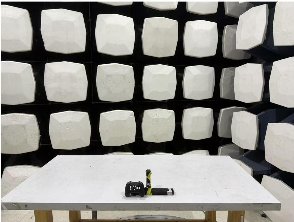
9KHz to 30MHz (EUT was placed in the centre of the turntable)
