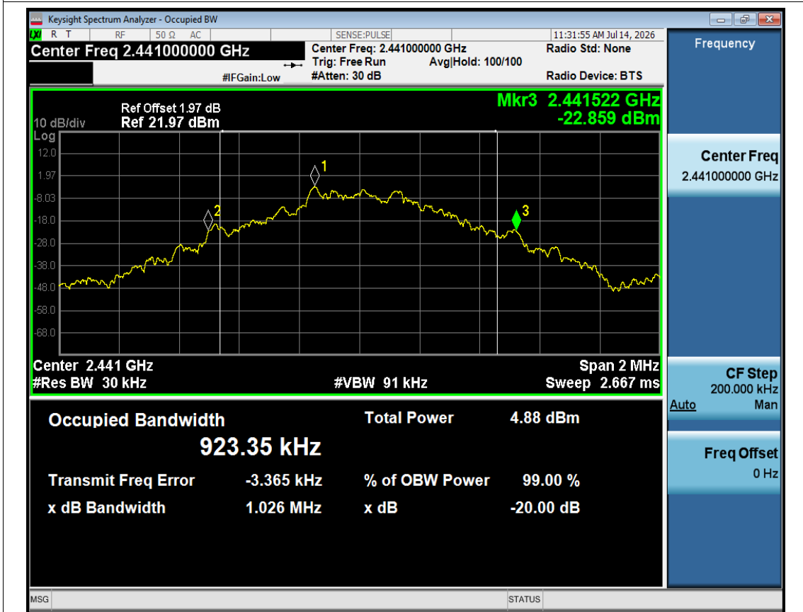
-20dB Bandwidth NVNT 1-DH1 2441MHz Ant1
