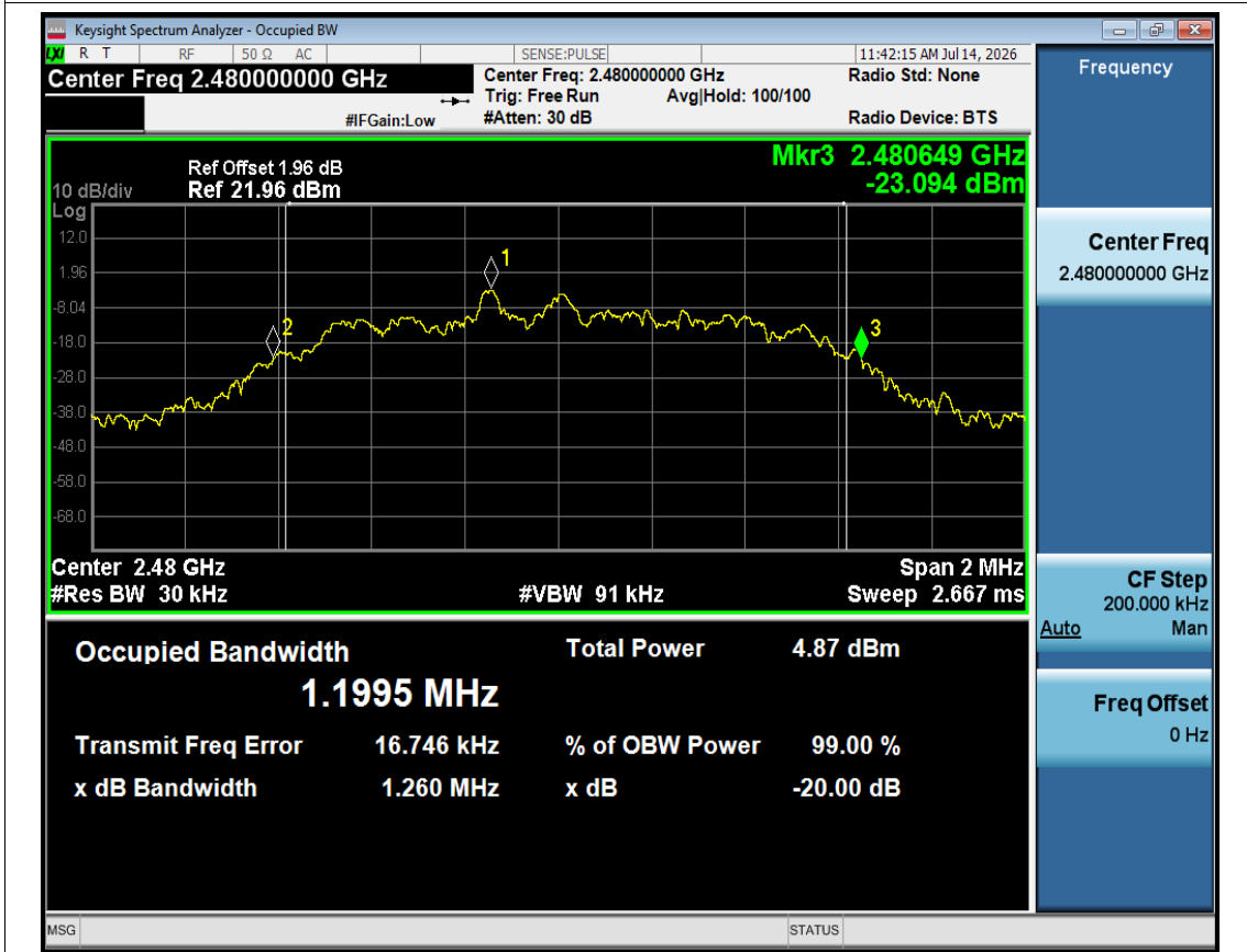
-20dB Bandwidth NVNT 2-DH1 2480MHz Ant1
