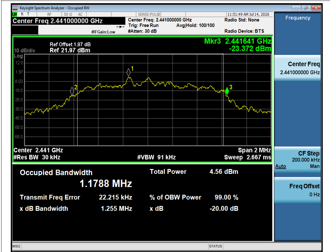
-20dB Bandwidth NVNT 3-DH1 2441MHz Ant1
