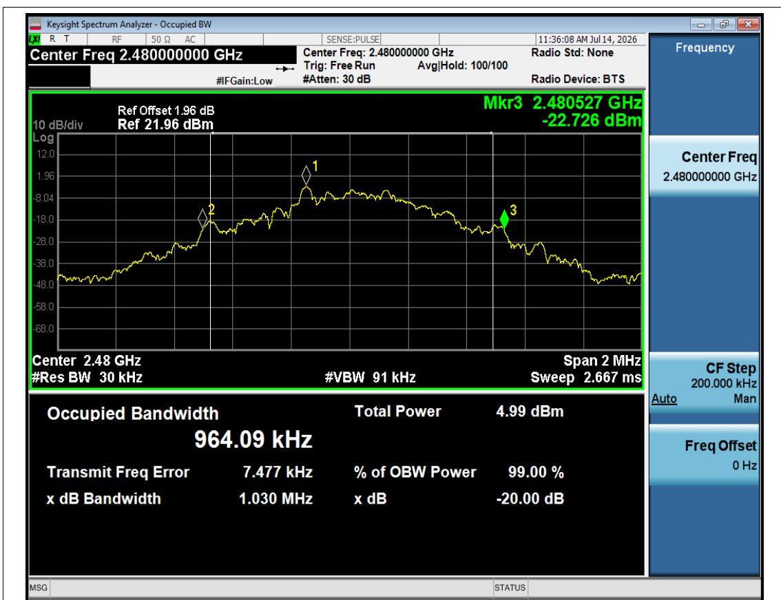
-20dB Bandwidth NVNT 1-DH1 2480MHz Ant1
