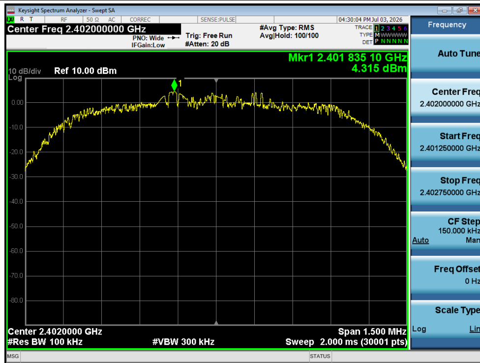
Tx. Spurious NVNT 3-DH5 2402MHz Ant1 Ref
