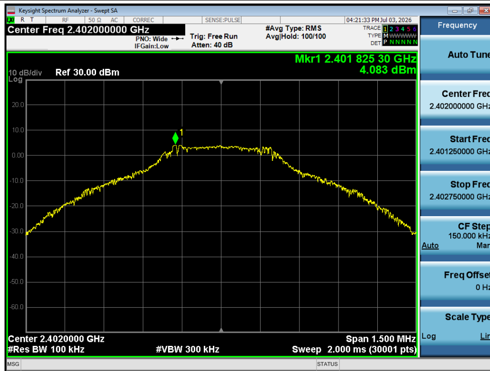
Tx. Spurious NVNT 1-DH5 2402MHz Ant1 Ref
