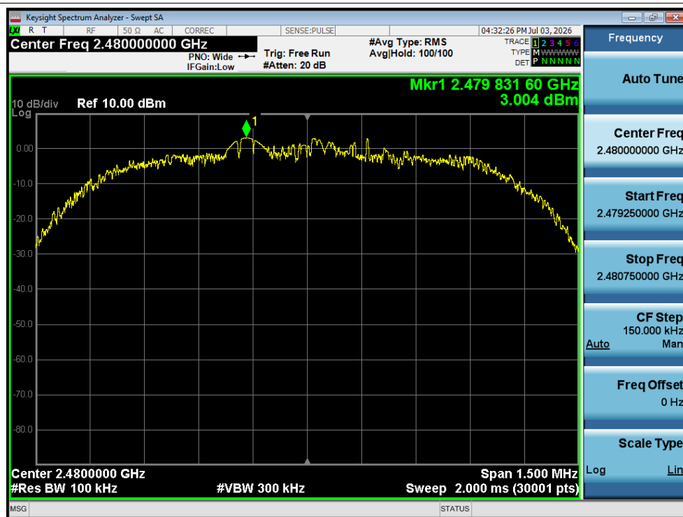
Tx. Spurious NVNT 3-DH5 2480MHz Ant1 Ref
