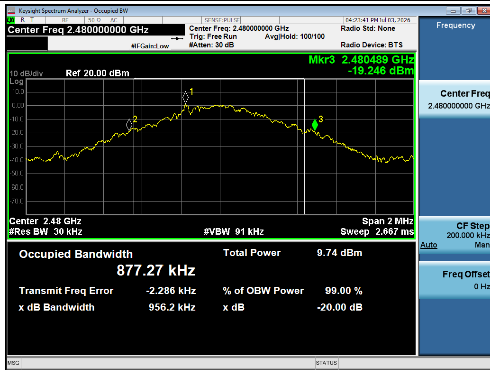
-20dB Bandwidth NVNT 1-DH5 2480MHz Ant1
