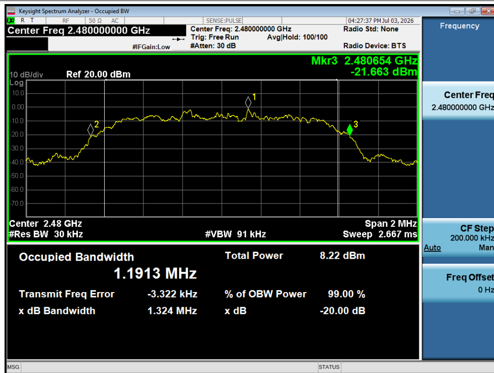
-20dB Bandwidth NVNT 2-DH5 2480MHz Ant1
