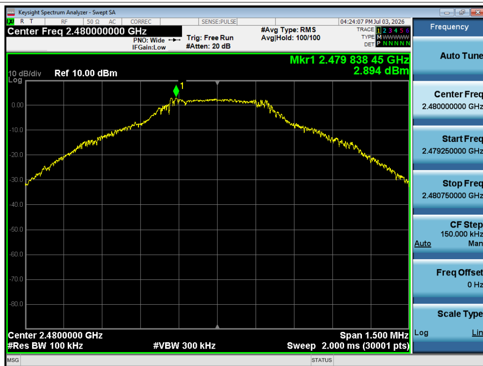
Tx. Spurious NVNT 1-DH5 2480MHz Ant1 Ref
