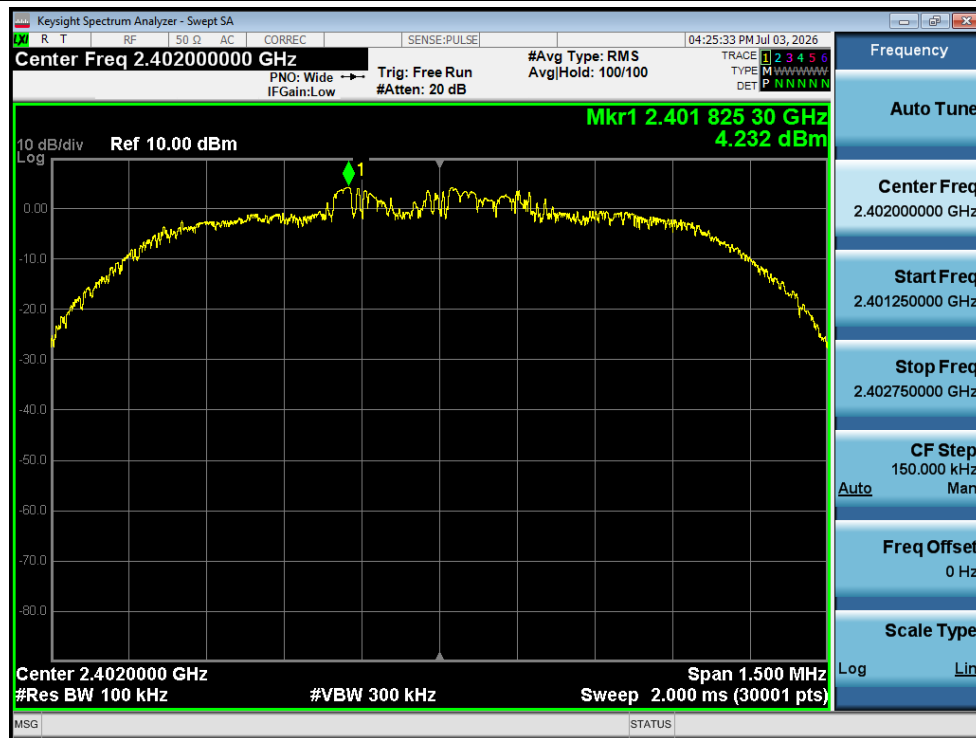
Tx. Spurious NVNT 2-DH5 2402MHz Ant1 Ref
