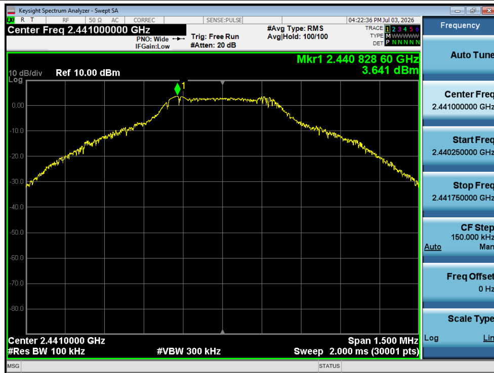
Tx. Spurious NVNT 1-DH5 2441MHz Ant1 Ref
