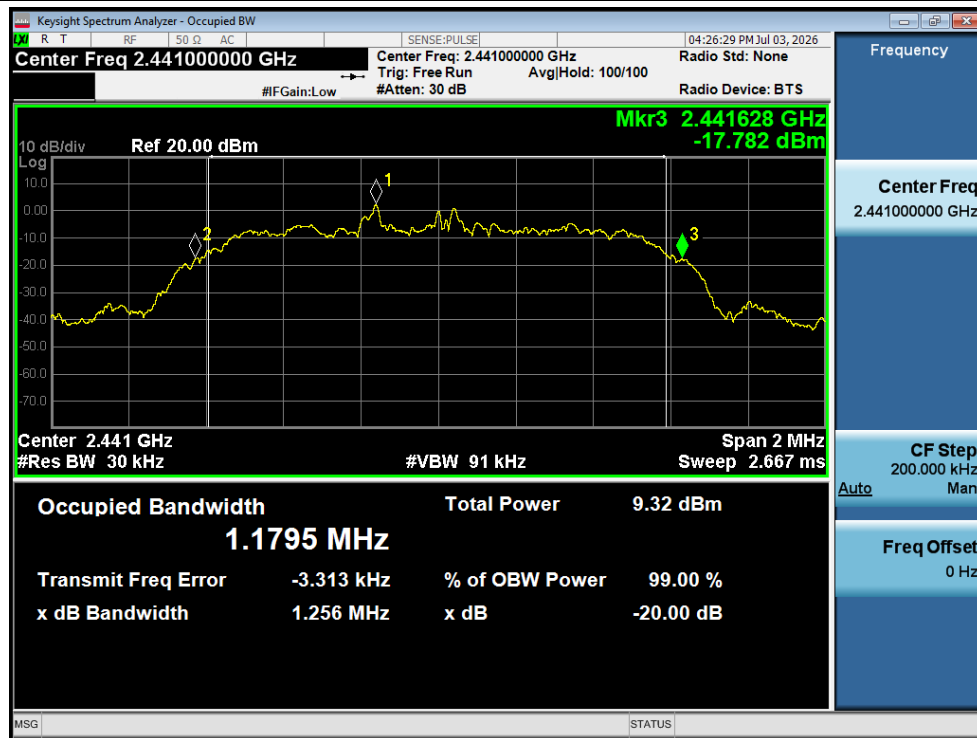
-20dB Bandwidth NVNT 2-DH5 2441MHz Ant1
