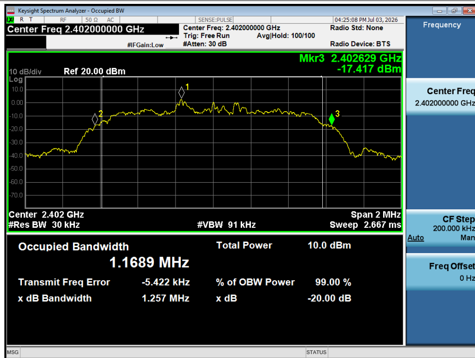
-20dB Bandwidth NVNT 2-DH5 2402MHz Ant1
