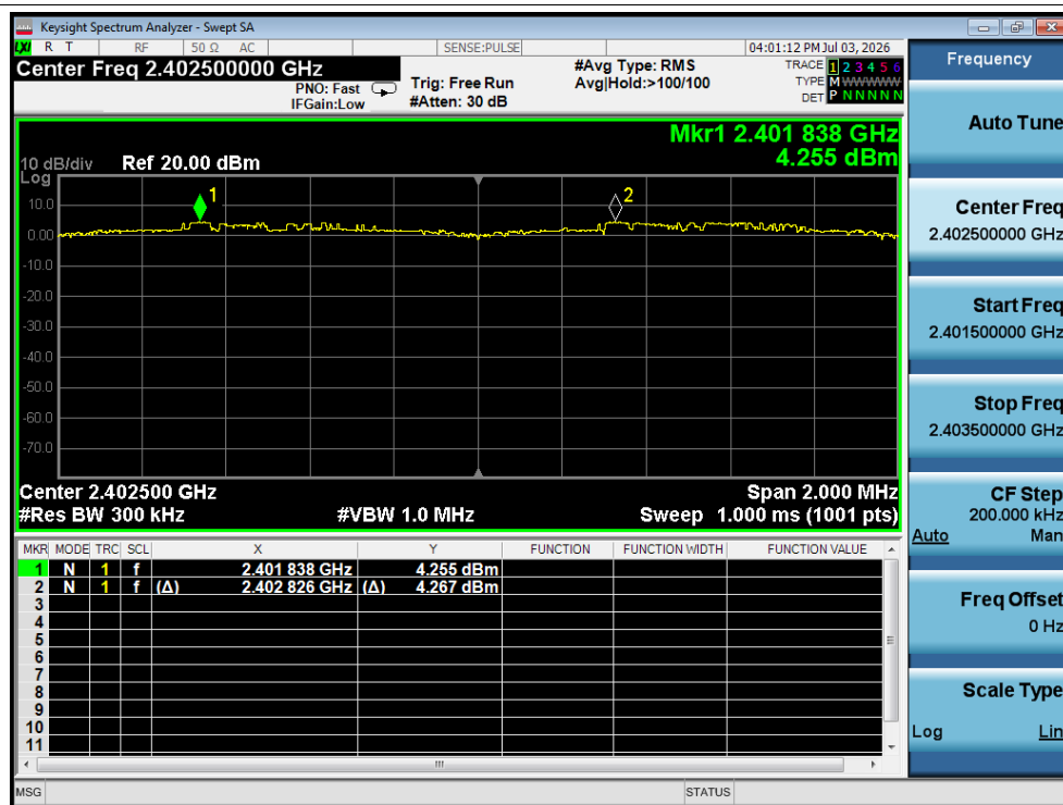
CFS NVNT 2-DH5 2402MHz Ant1
