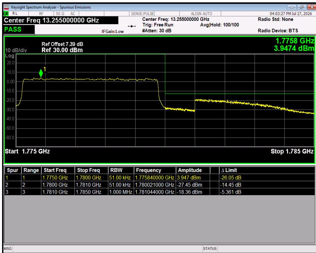
Band66 16QAM BW=5MHz Channel=132647 RB Size=1 Position=#0
