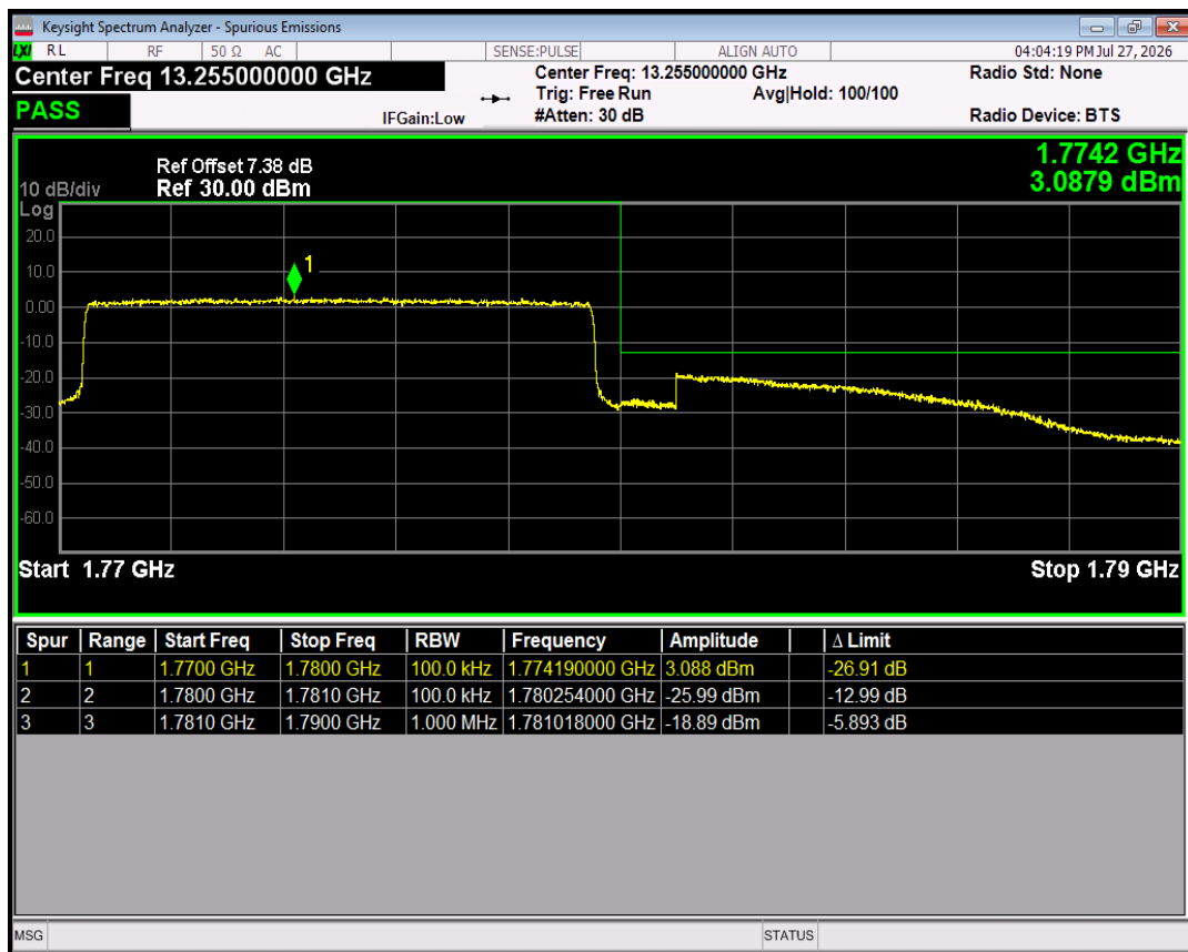
Band66 16QAM BW=10MHz Channel=132622 RB Size=1 Position=#0
