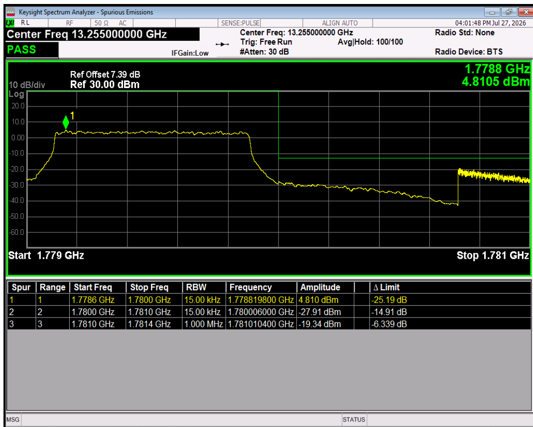
Band66 16QAM BW=1.4MHz Channel=132665 RB Size=1 Position=#0
