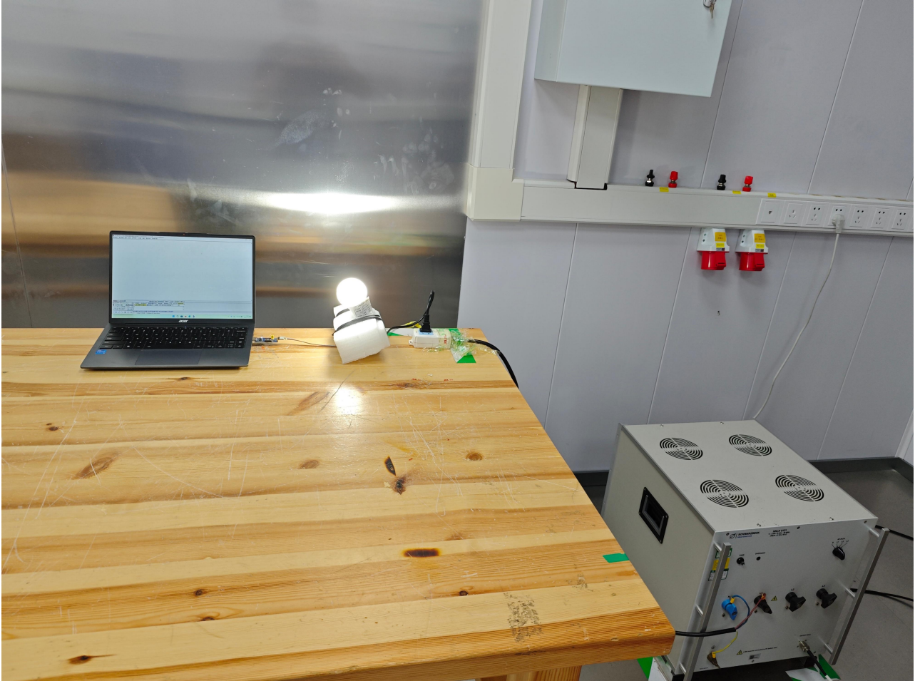
AC Power Line Conducted Emissions Test View
