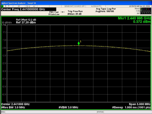
Peak Output Power 8DPSK Channel 39
