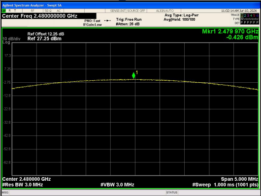
Peak Output Power 8DPSK Channel 78
