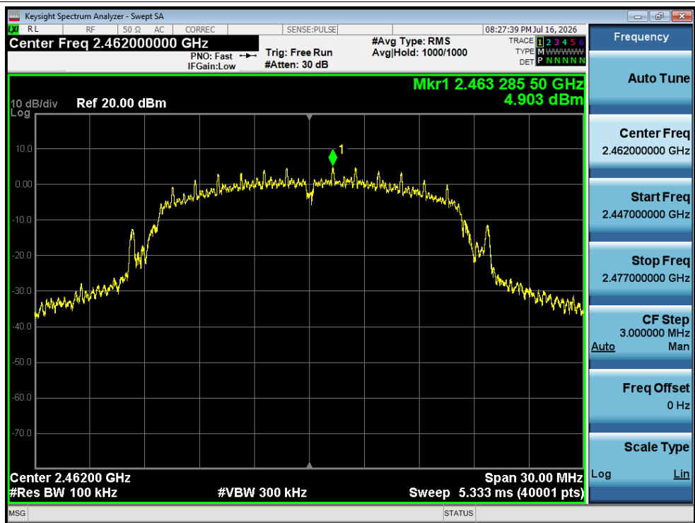
Tx. Spurious NVNT g 2462MHz Ant1 Ref
