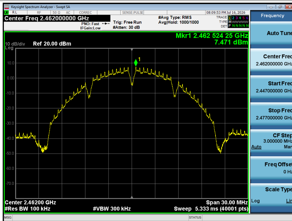
Tx. Spurious NVNT b 2462MHz Ant1 Ref
