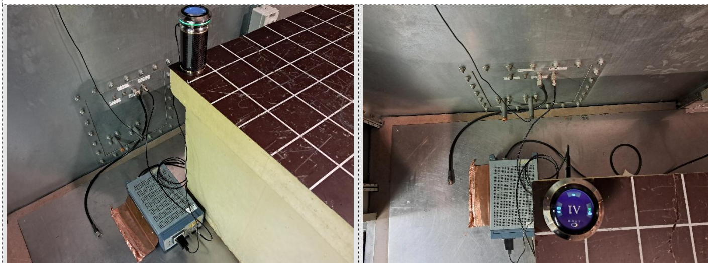
PHOTO N°4 - CONDUCTED EMISSION TEST SETUP
