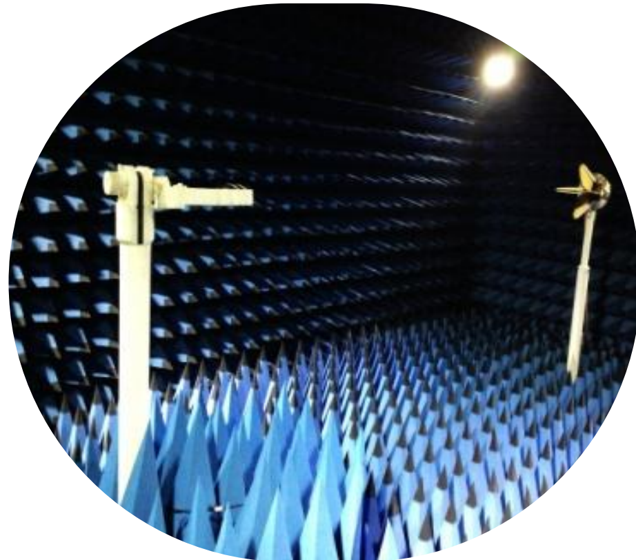
7m x 4m x 3m microwave anechoic chamber
