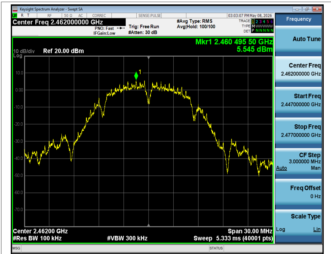
Tx. Spurious NVNT b 2462MHz Ant1 Ref
