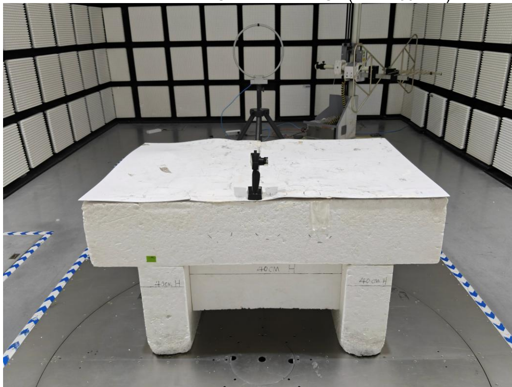
RADIATED RF MEASUREMENT SETUP (Below 30MHz)
