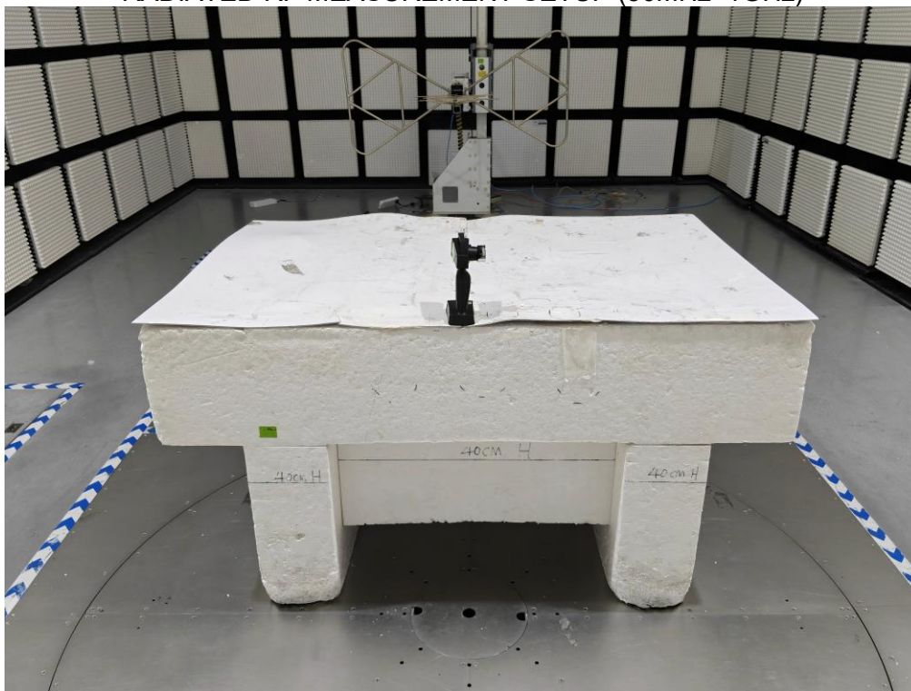
RADIATED RF MEASUREMENT SETUP (30MHz~1GHz)
