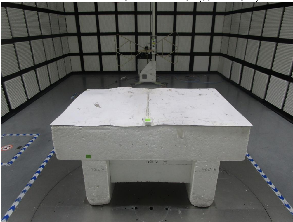
RADIATED RF MEASUREMENT SETUP (30MHz~1GHz)
