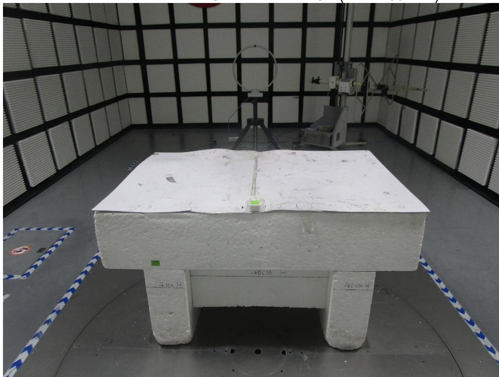
RADIATED RF MEASUREMENT SETUP (Below 30MHz)
