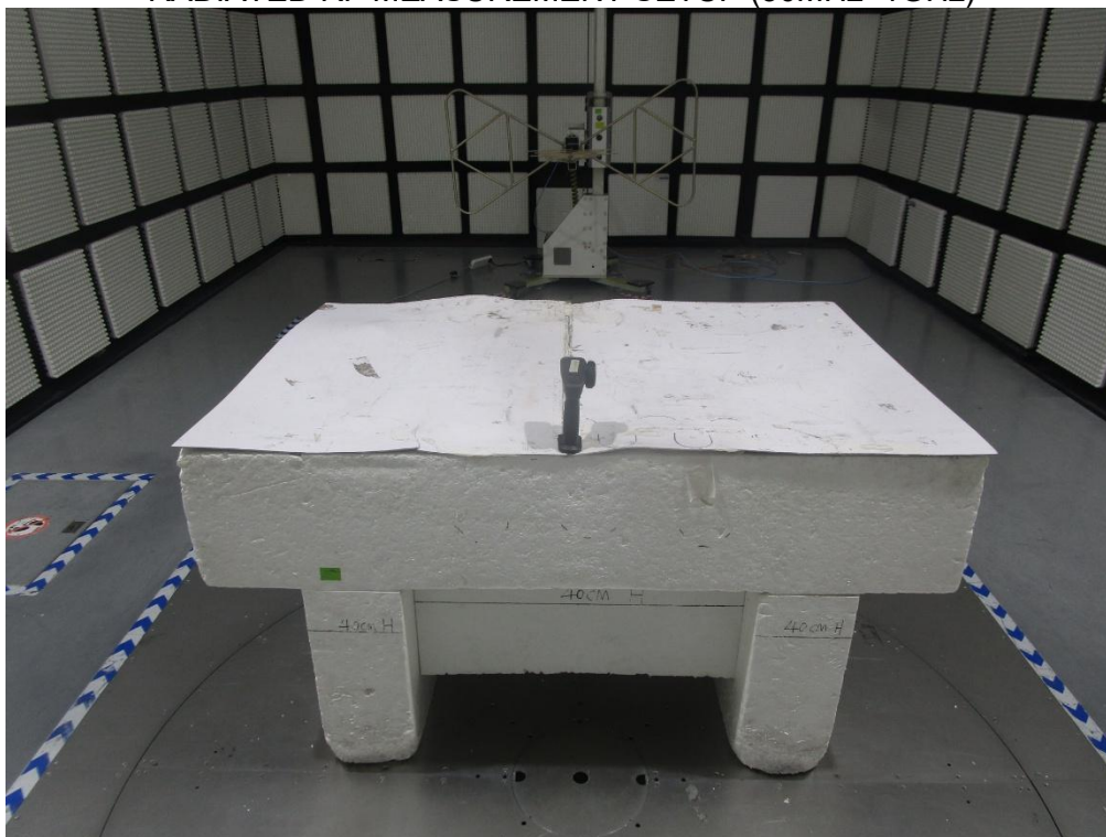
RADIATED RF MEASUREMENT SETUP (30MHz~1GHz)
