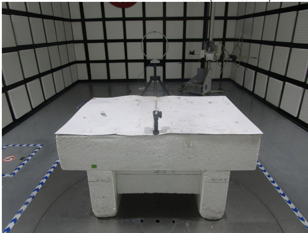
RADIATED RF MEASUREMENT SETUP (Below 30MHz)
