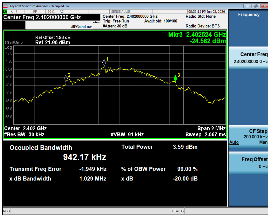
-20dB Bandwidth NVNT 1-DH1 2402MHz Ant1
