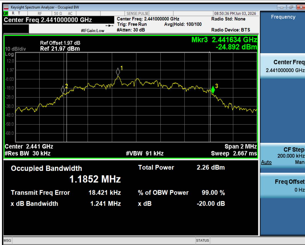
-20dB Bandwidth NVNT 3-DH1 2441MHz Ant1
