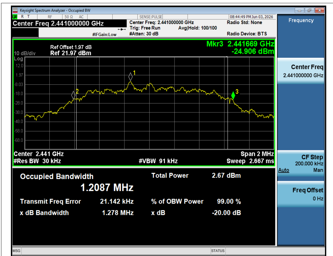
-20dB Bandwidth NVNT 2-DH1 2441MHz Ant1
