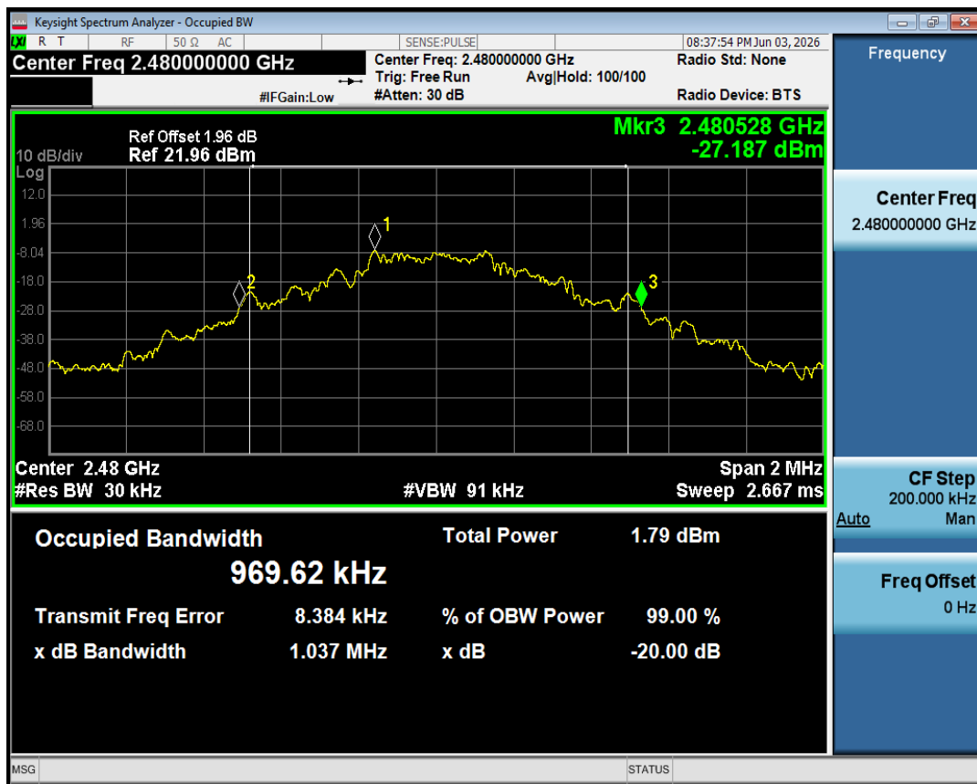
-20dB Bandwidth NVNT 1-DH1 2480MHz Ant1
