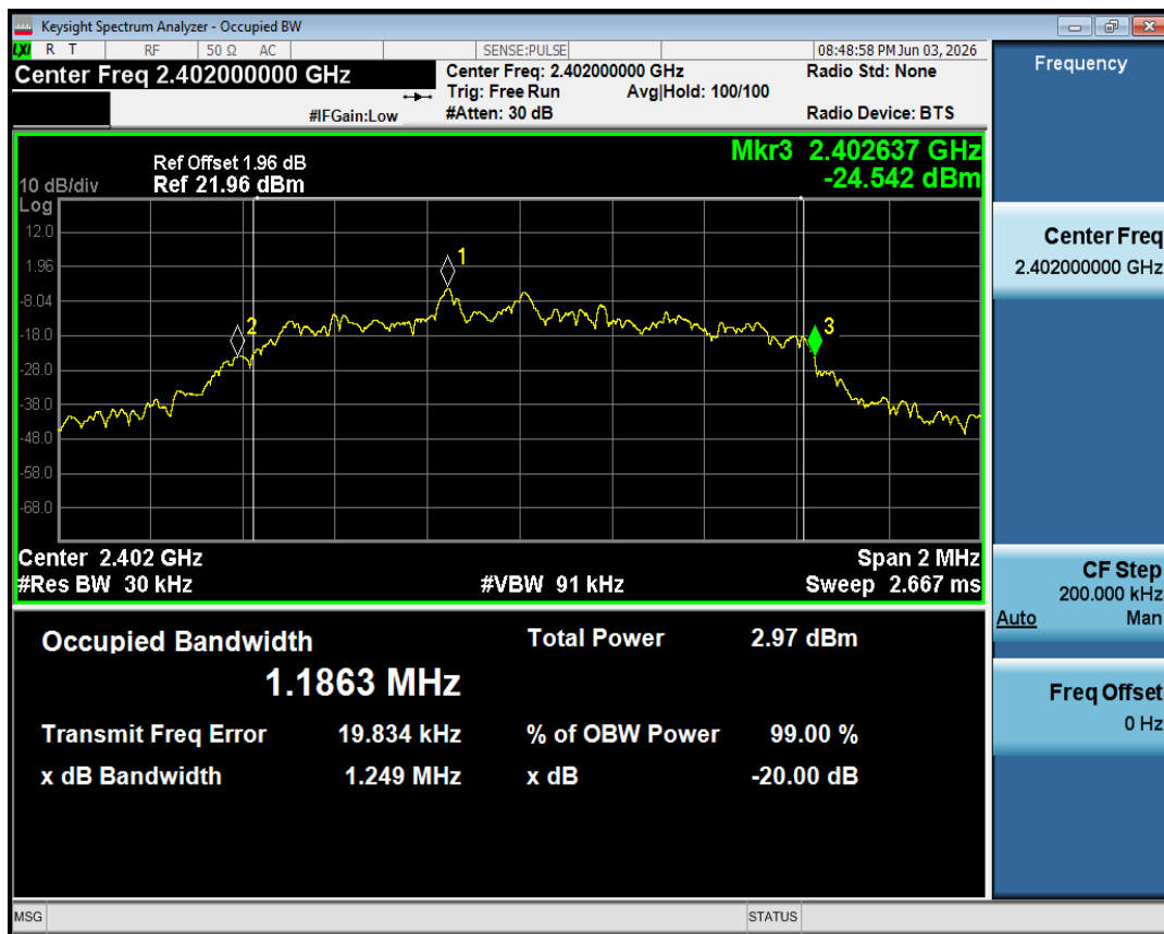
-20dB Bandwidth NVNT 3-DH1 2402MHz Ant1
