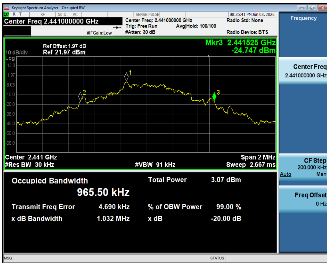
-20dB Bandwidth NVNT 1-DH1 2441MHz Ant1
