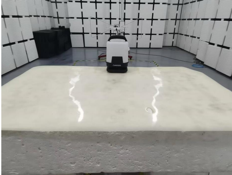
Set-up for Radiated Spurious Emission, Above 1GHz
