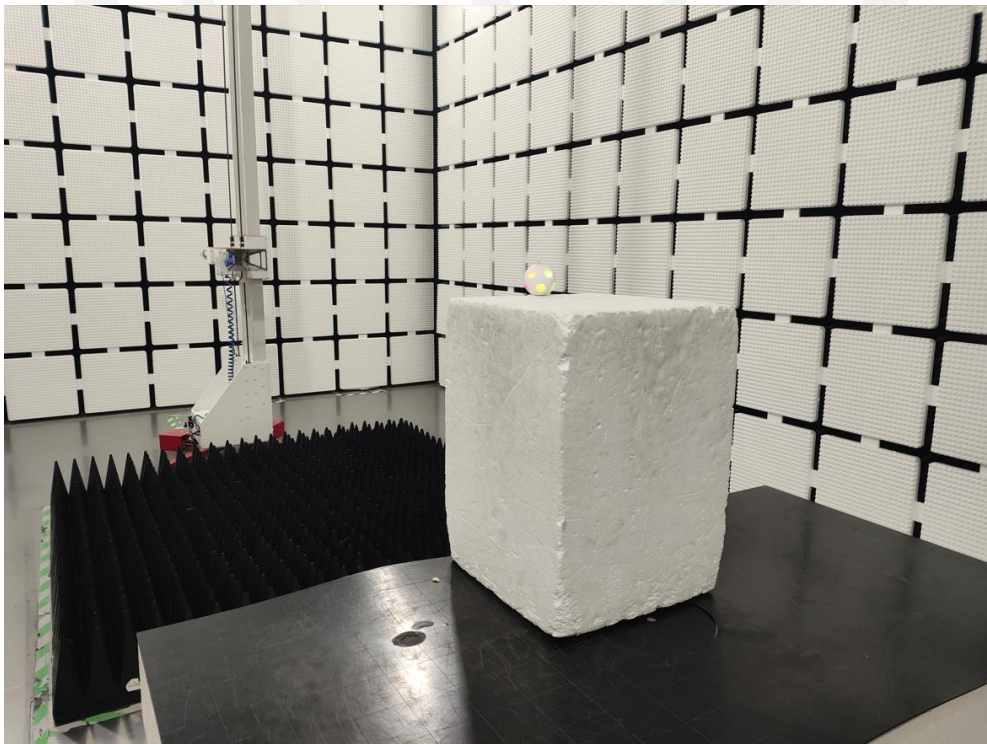
Spurious Radiation Emissions Test (>1G)
