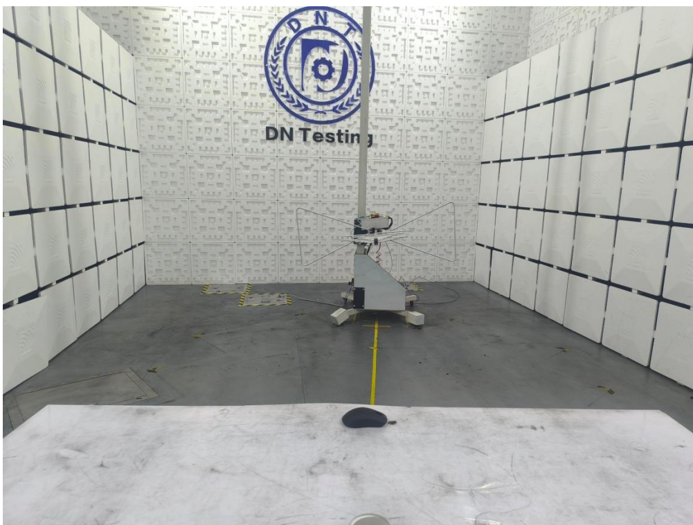
Radiated Emission Test View|(Below 1G)
