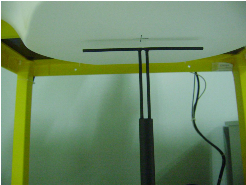
Setup Photo of Dipole Antenna
