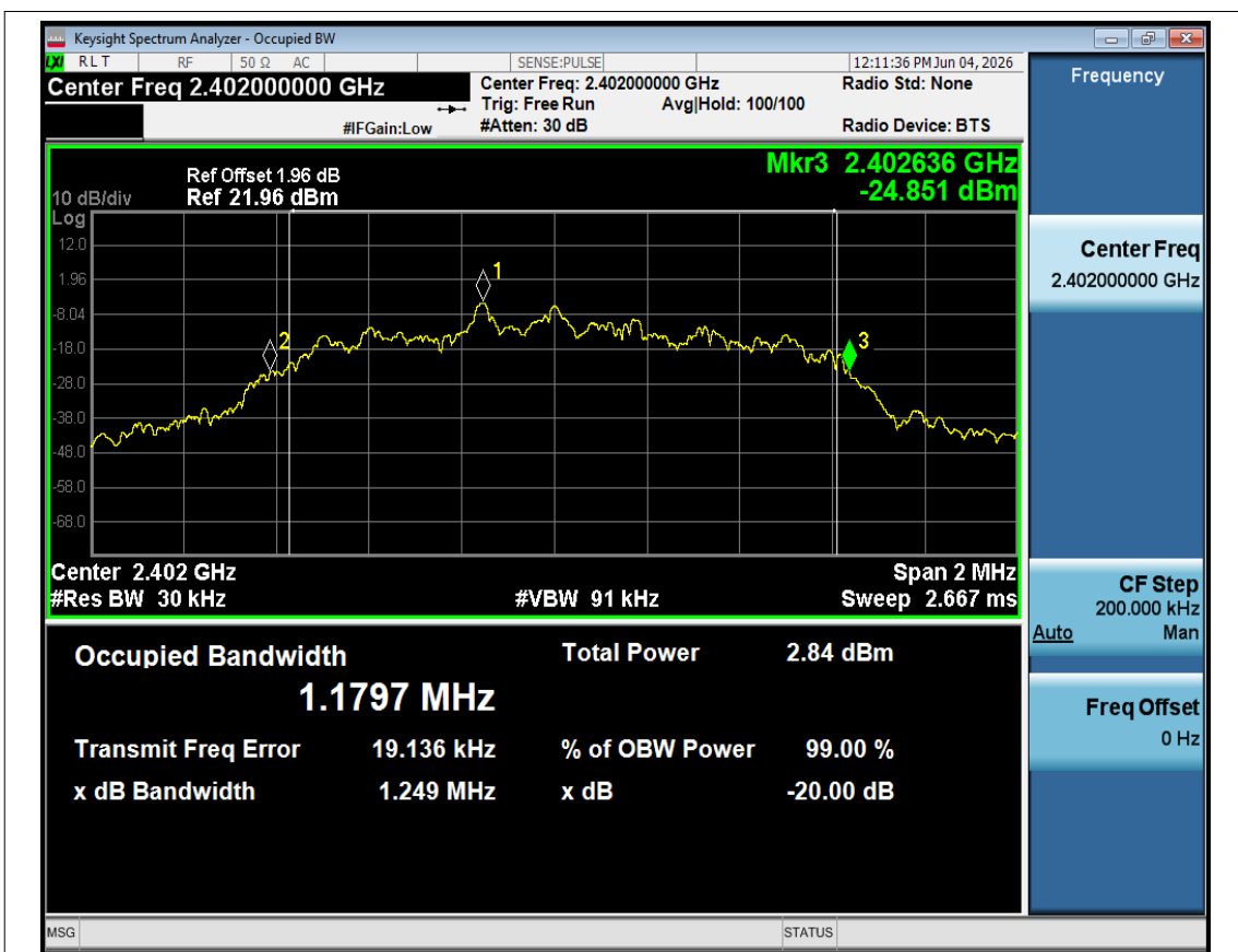
-20dB Bandwidth NVNT 3-DH1 2402MHz Ant1
