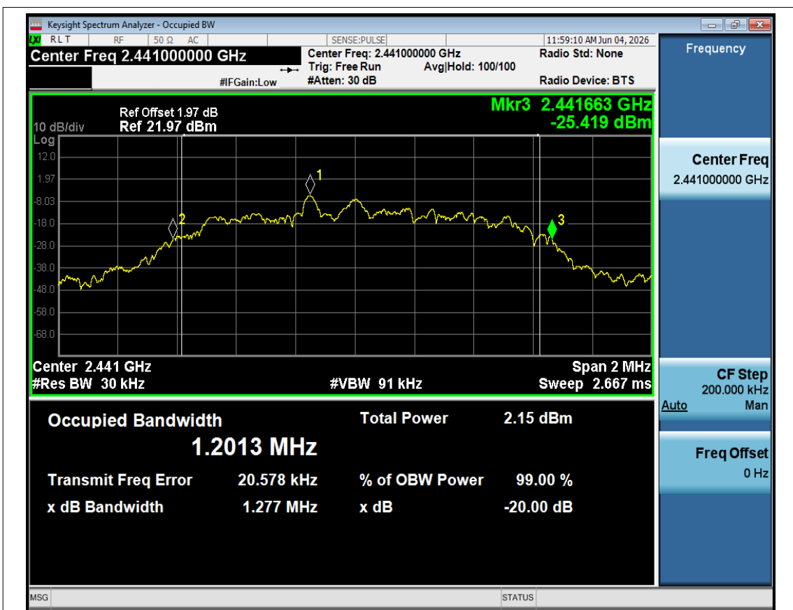
-20dB Bandwidth NVNT 2-DH1 2441MHz Ant1
