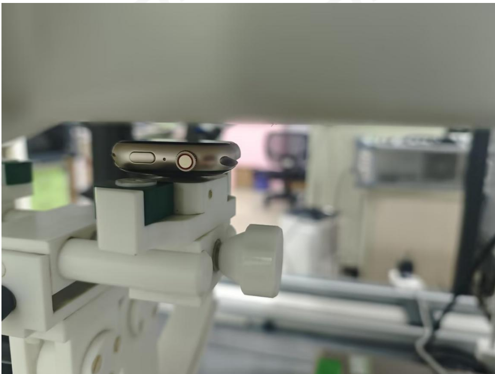
Front of face (separation distance is 10mm)
