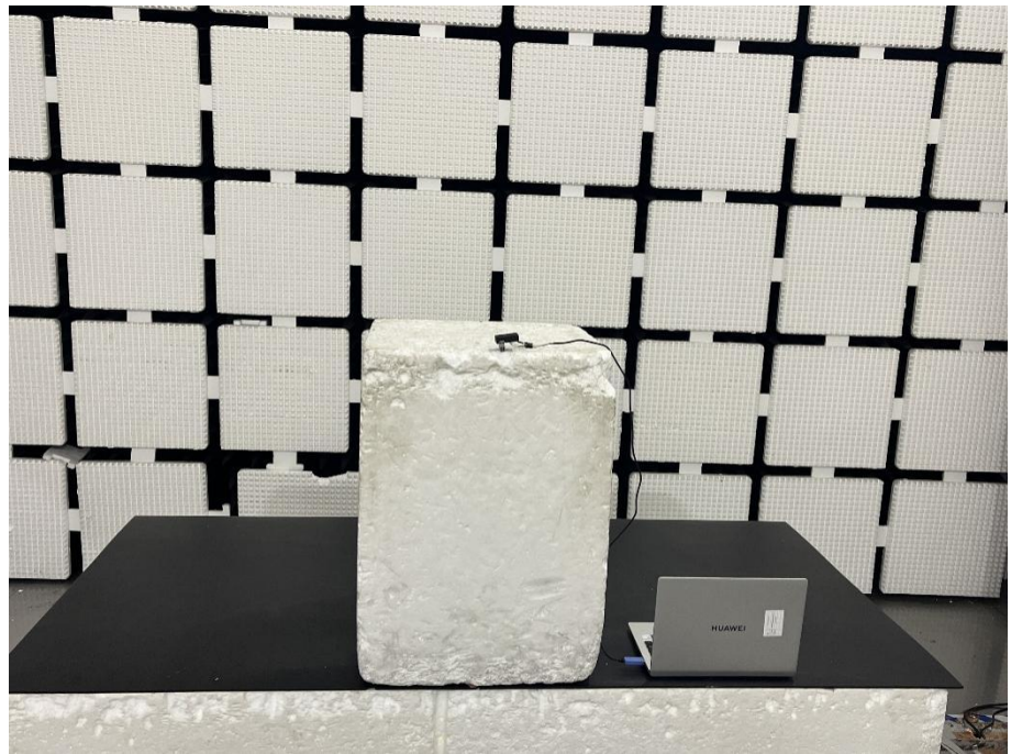
Radiation Emission Test Setup (close up)
