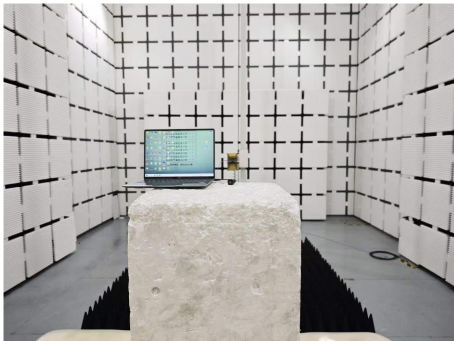
Set-up for Radiated Spurious Emission, Above 1GHz
