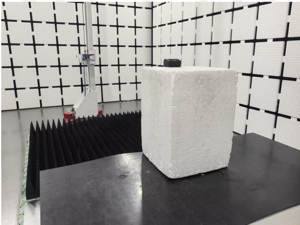
Spurious Radiation Emissions Test (>1G)
