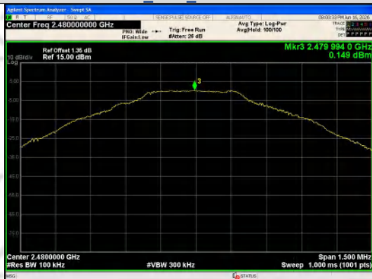
In-Band Reference Level GFSK DH5 Channel 78
