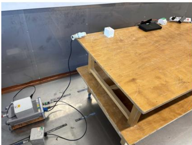
Photo of AC Power Line Conducted Emissions
