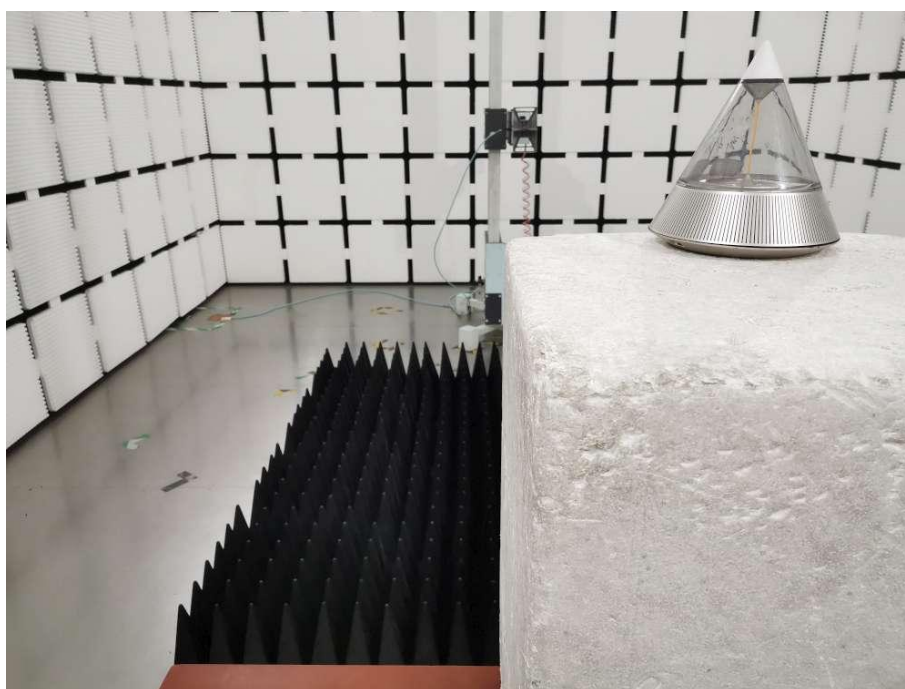
Radiated Emission Test View 2
