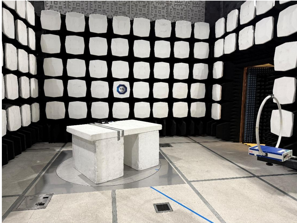
Figure 1 – Test Set up Front View - Radiated Emissions <30 MHz - coaxial
