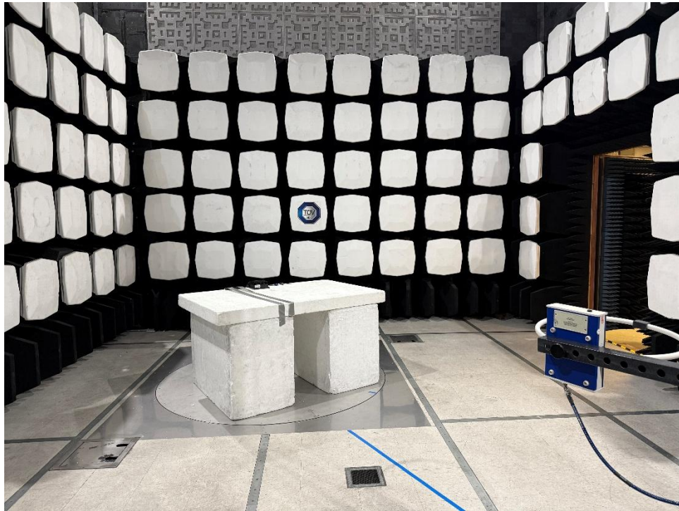
Figure 5 – Test Set up Front View - Radiated Emissions <30 MHz - coplanar horizontal
