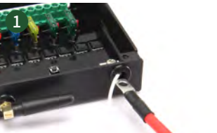
Insert the positive and negative poles into the corresponding holes
