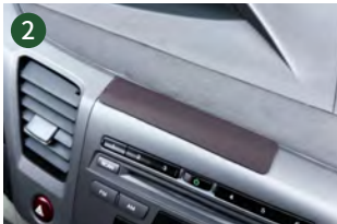
Attach the magnetic sheet to the car surface
