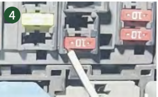
The white line connects to the original car's insurance (Electricity only comes after starting the car)
