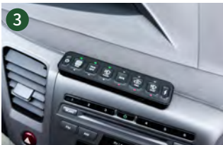
Attach the switch to the magnetic plate
