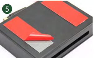
Double sided adhesive film torn off
