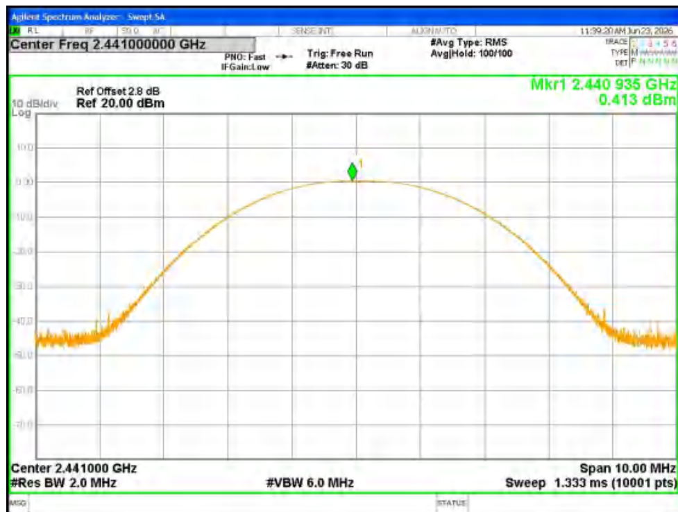
Peak Power NVNT 1-DH5 2441MHz Ant1
