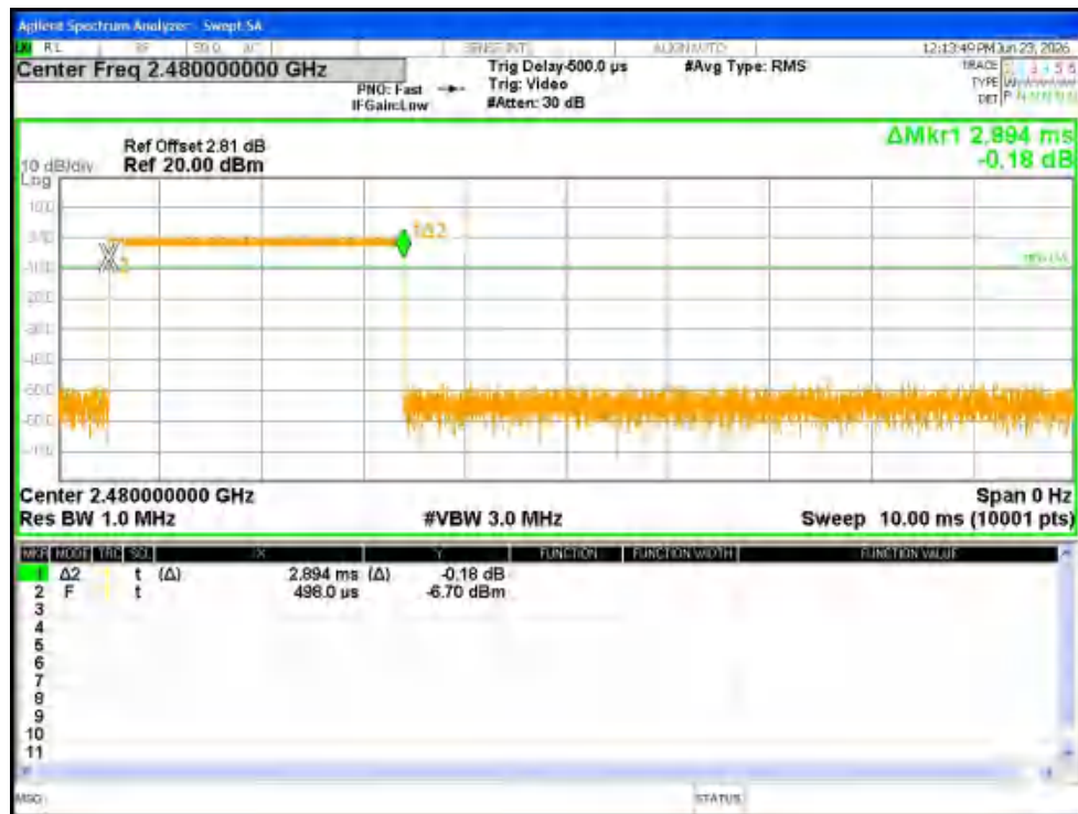
Dwell NVNT 3-DH5 2480MHz Ant1 One Burst
