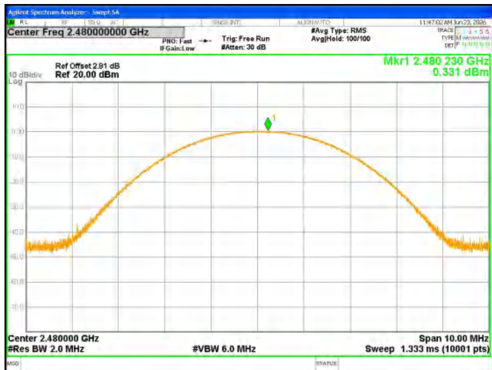
Peak Power NVNT 2-DH5 2480MHz Ant1
