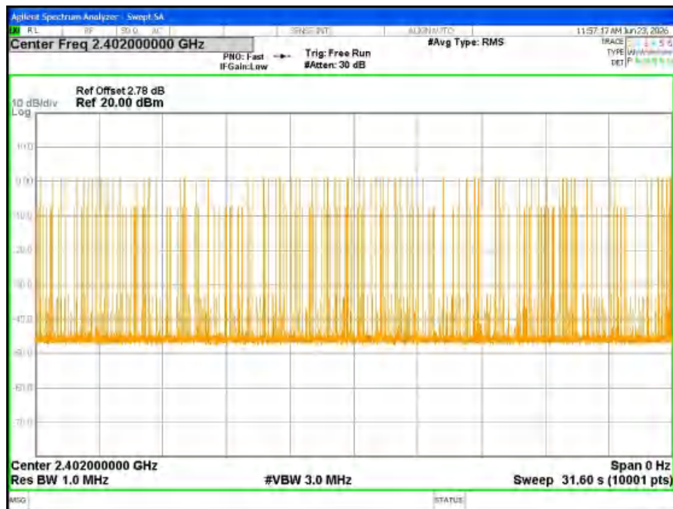
Dwell NVNT 1-DH5 2402MHz Ant1 Accumulated
