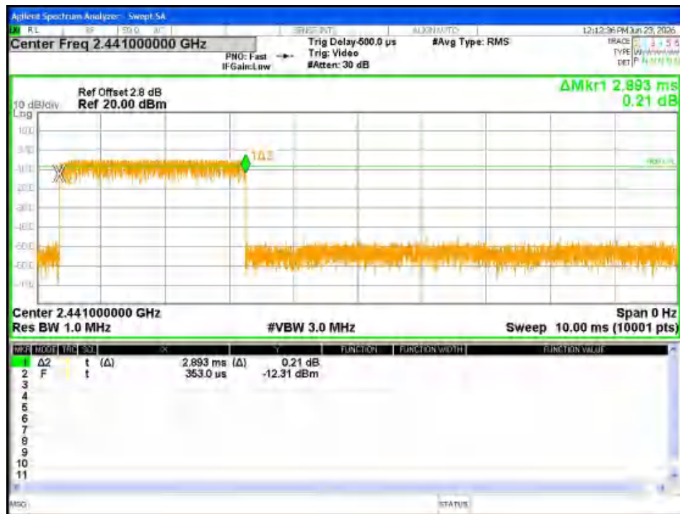
Dwell NVNT 3-DH5 2441MHz Ant1 One Burst
