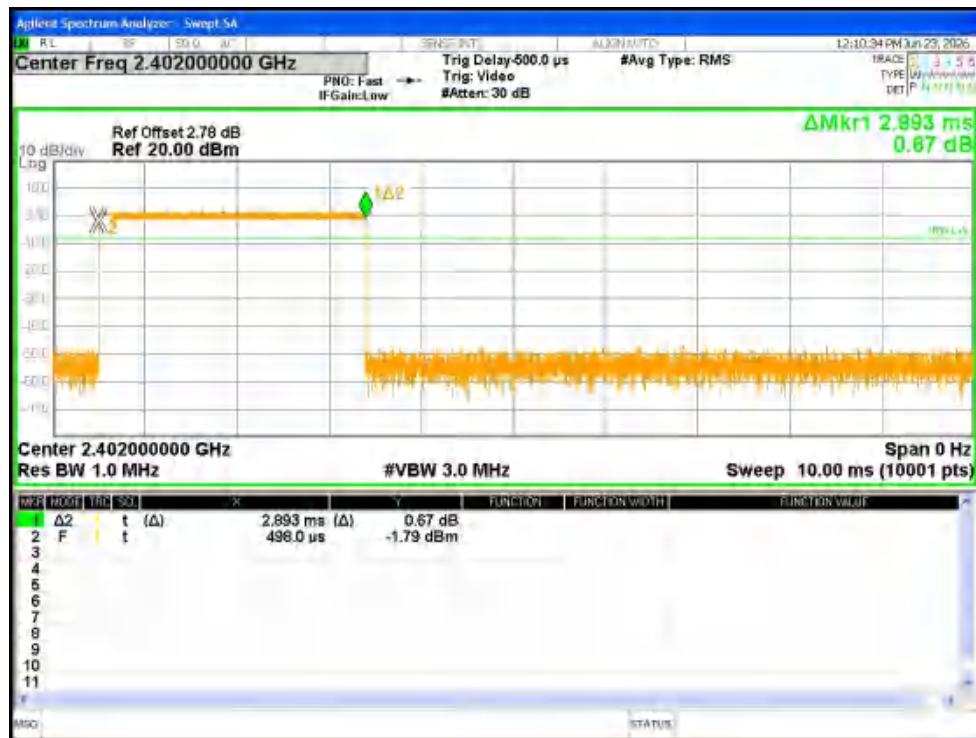
Dwell NVNT 3-DH5 2402MHz Ant1 One Burst
