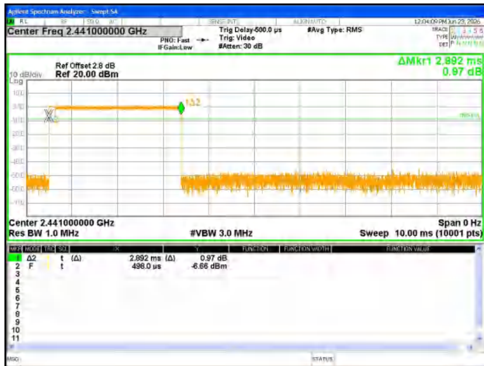
Dwell NVNT 2-DH5 2441MHz Ant1 One Burst
