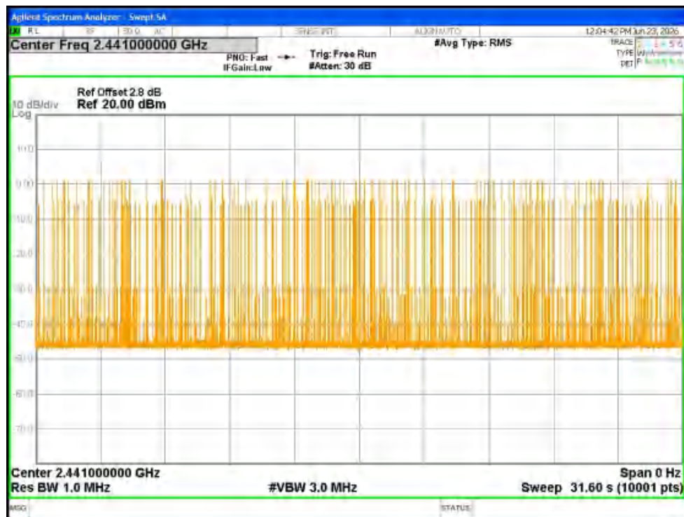
Dwell NVNT 2-DH5 2441MHz Ant1 Accumulated
