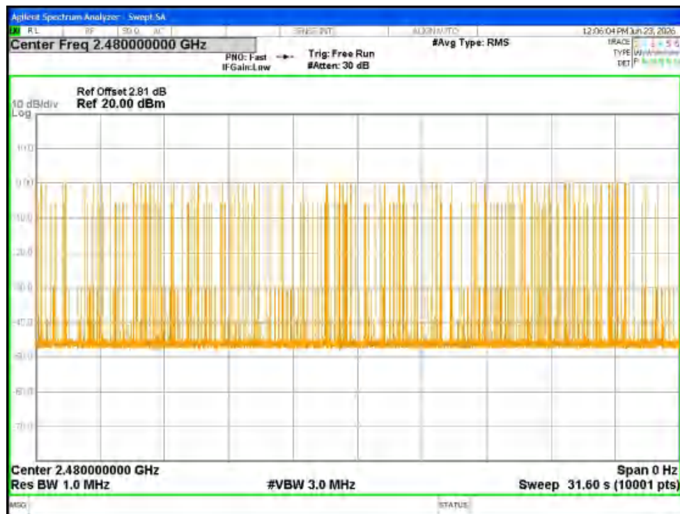
Dwell NVNT 2-DH5 2480MHz Ant1 Accumulated
