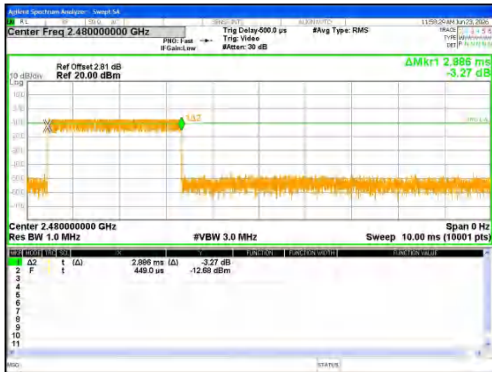
Dwell NVNT 1-DH5 2480MHz Ant1 One Burst
