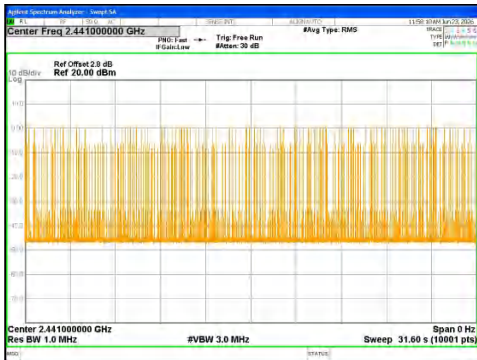
Dwell NVNT 1-DH5 2441MHz Ant1 Accumulated
