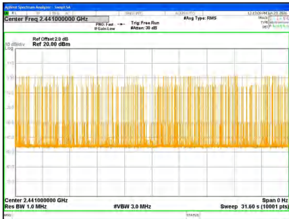
Dwell NVNT 3-DH5 2441MHz Ant1 Accumulated
