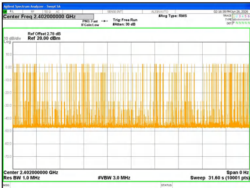
Dwell NVNT 2-DH5 2402MHz Ant1 Accumulated
