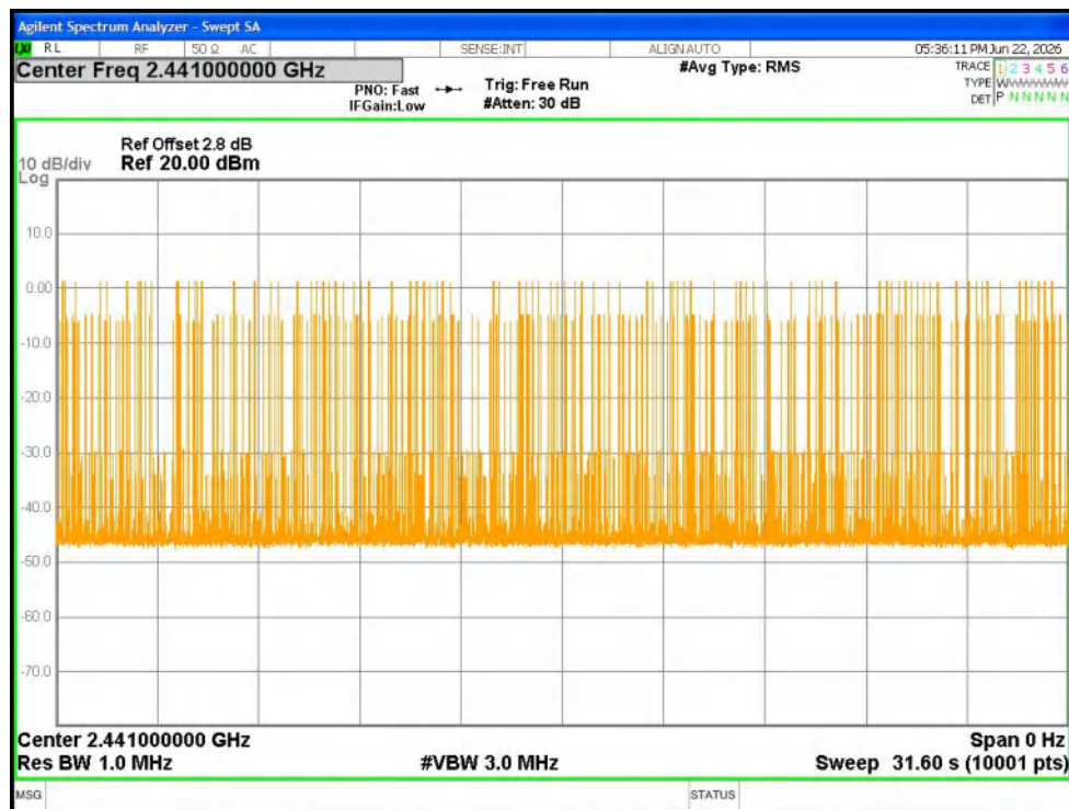
Dwell NVNT 3-DH5 2441MHz Ant1 Accumulated
