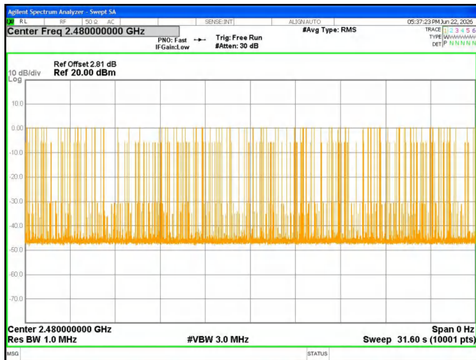
Dwell NVNT 3-DH5 2480MHz Ant1 Accumulated
