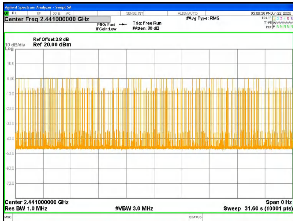
Dwell NVNT 1-DH5 2441MHz Ant1 Accumulated
