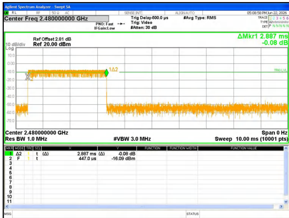
Dwell NVNT 1-DH5 2480MHz Ant1 One Burst
