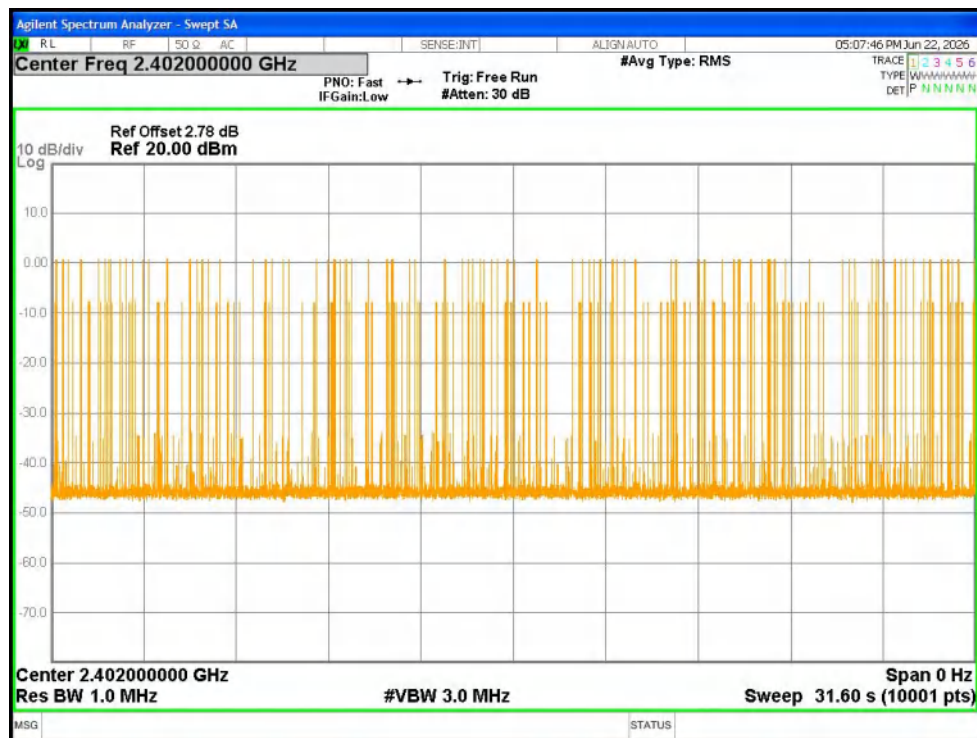
Dwell NVNT 1-DH5 2402MHz Ant1 Accumulated
