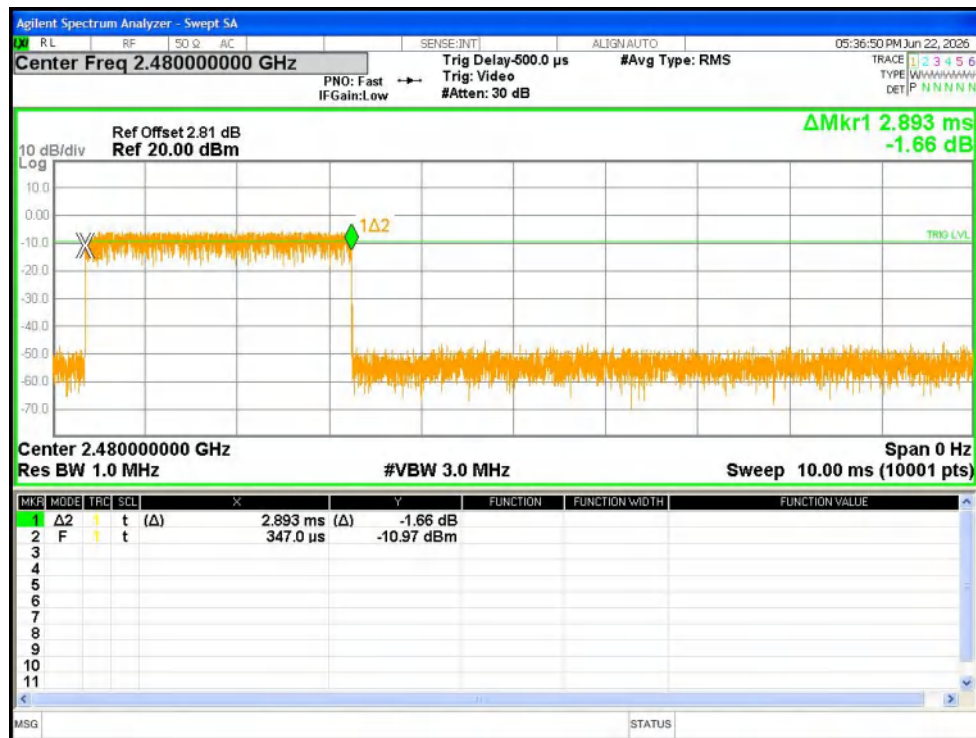
Dwell NVNT 3-DH5 2480MHz Ant1 One Burst
