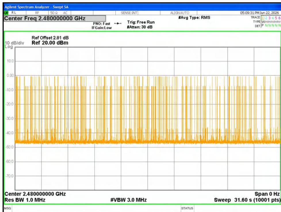
Dwell NVNT 1-DH5 2480MHz Ant1 Accumulated
