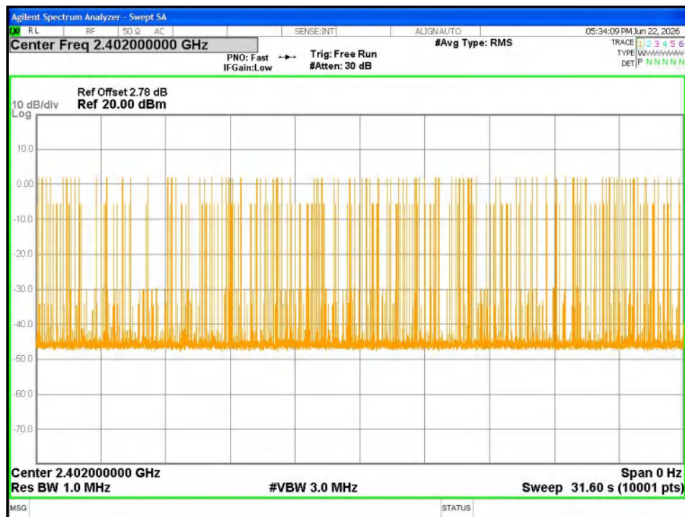
Dwell NVNT 3-DH5 2402MHz Ant1 Accumulated
