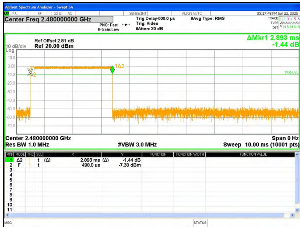
Dwell NVNT 2-DH5 2480MHz Ant1 One Burst
