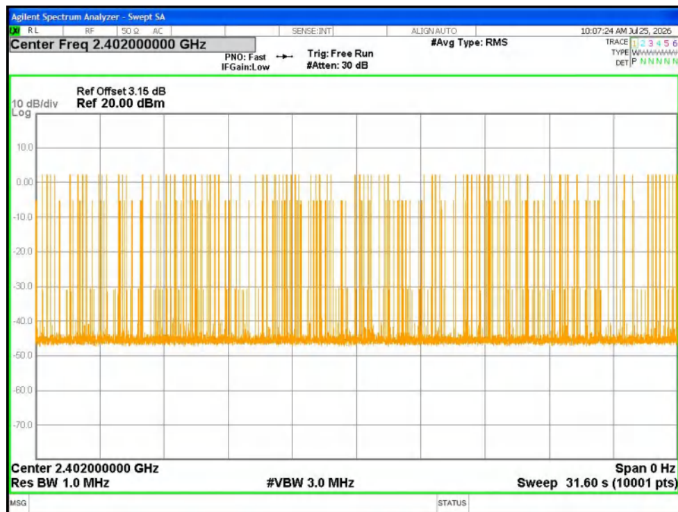
Dwell NVNT 3-DH5 2402MHz Ant1 Accumulated
