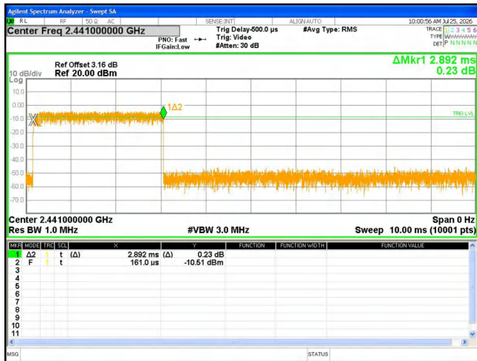
Dwell NVNT 2-DH5 2441MHz Ant1 One Burst
