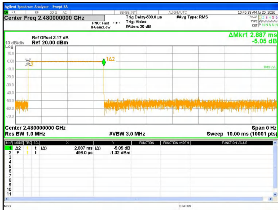
Dwell NVNT 1-DH5 2480MHz Ant1 One Burst
