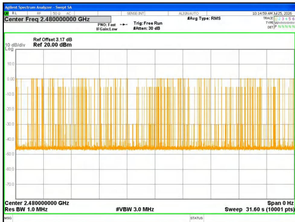
Dwell NVNT 2-DH5 2480MHz Ant1 Accumulated
