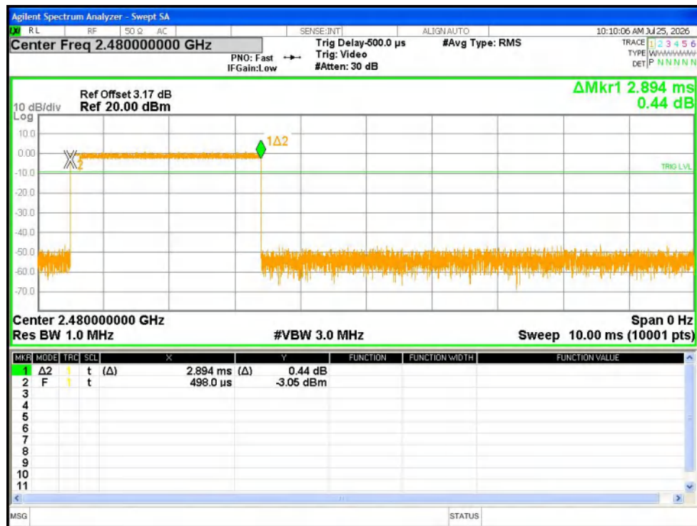
Dwell NVNT 3-DH5 2480MHz Ant1 One Burst
