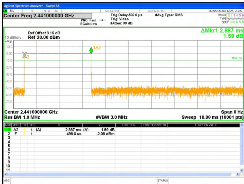
Dwell NVNT 1-DH5 2441MHz Ant1 One Burst
