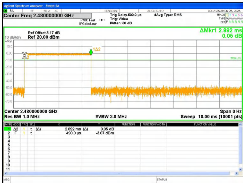
Dwell NVNT 2-DH5 2480MHz Ant1 One Burst
