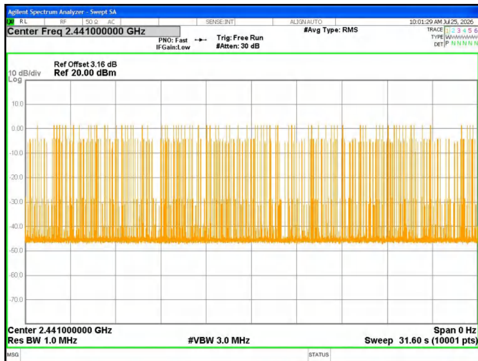
Dwell NVNT 2-DH5 2441MHz Ant1 Accumulated
