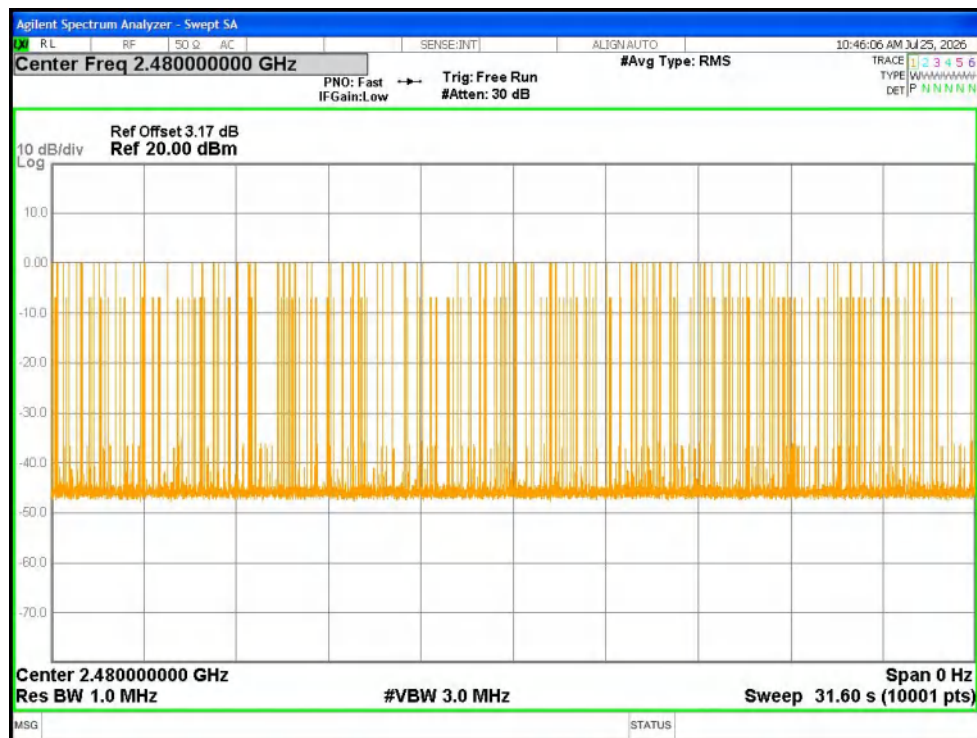
Dwell NVNT 1-DH5 2480MHz Ant1 Accumulated
