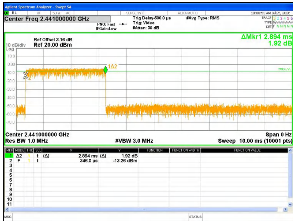
Dwell NVNT 3-DH5 2441MHz Ant1 One Burst
