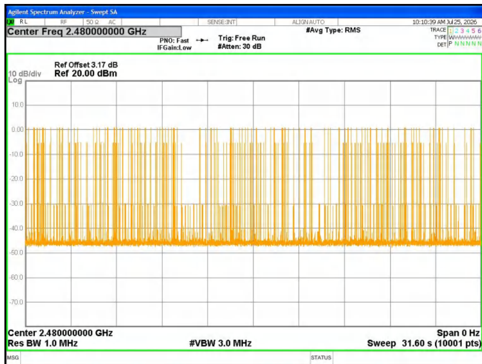
Dwell NVNT 3-DH5 2480MHz Ant1 Accumulated
