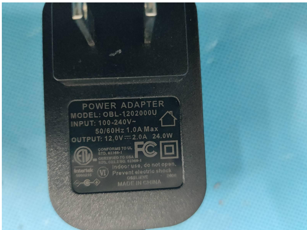
Adapter view of EUT
