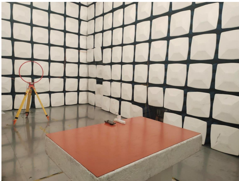
Radiated Emission below 30MHz-AC adapter charge mode
