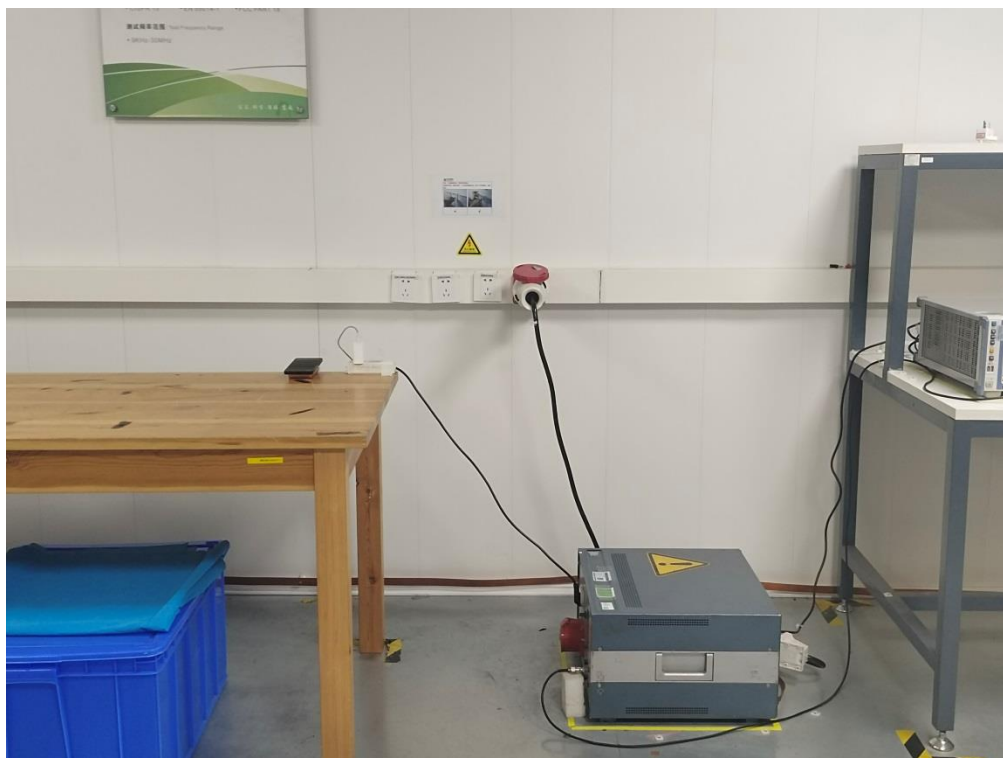
Conducted Emission-AC adapter charge mode
