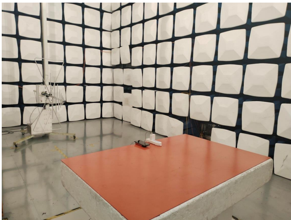
Radiated Emission below 1GHz-AC adapter charge mode
