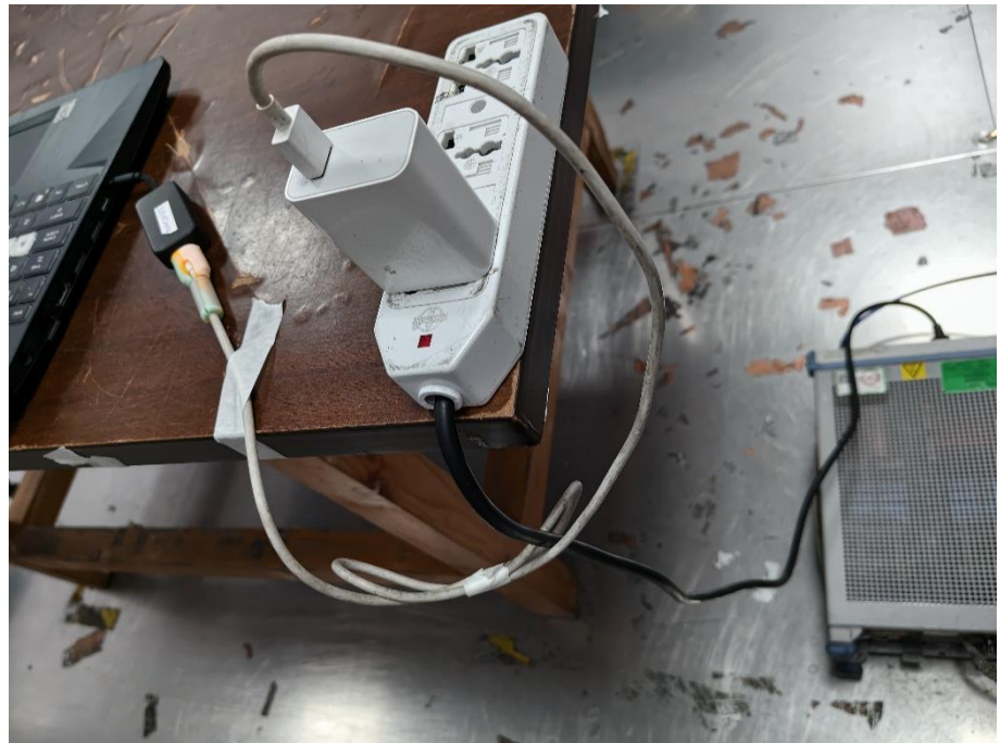
Conducted Emission Test Setup(close up)
