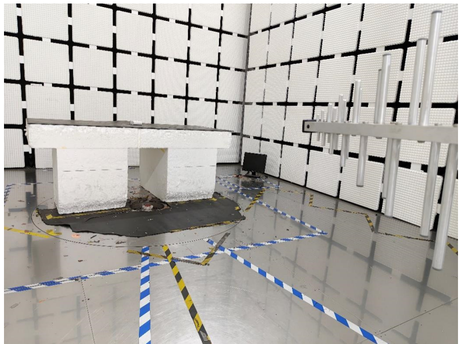
Radiation Emission Test Setup (30MHz to 1GHz)
